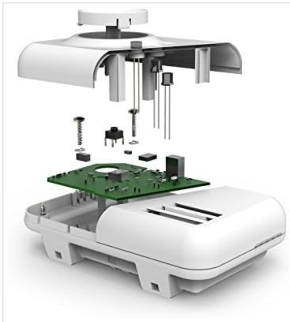
Figure 4: Exploded view of the FireAngel CO-9XT-FF Carbon Monoxide Alarm, showing internal components such as the circuit board and sensor.
