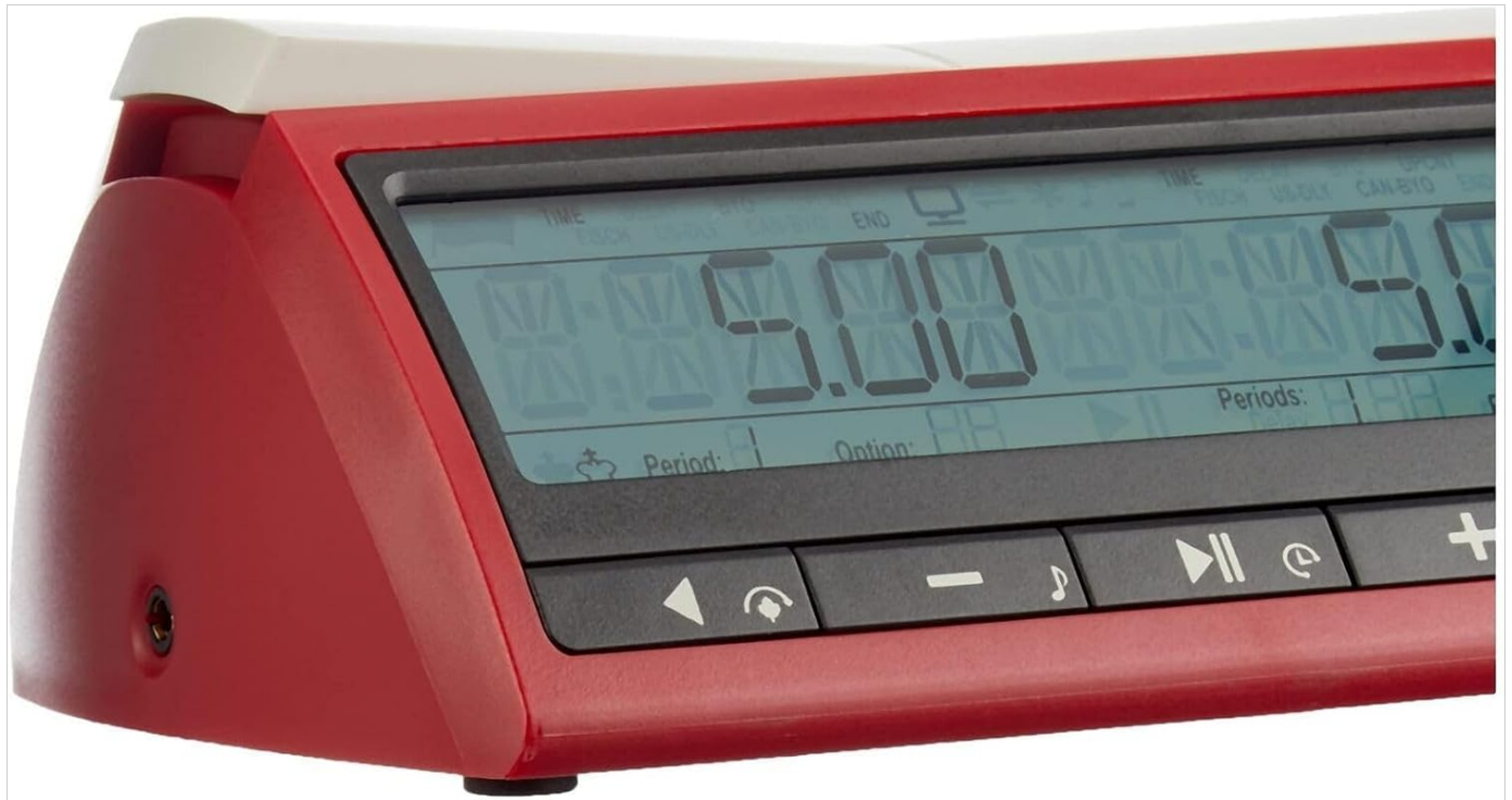
Figure 4.1: Side view of the DGT 3000, showing the power input port.
