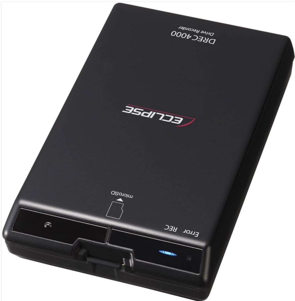
Image: An angled view of the DREC4000 main unit, illustrating the microSD card slot for easy removal and access to recorded data.
