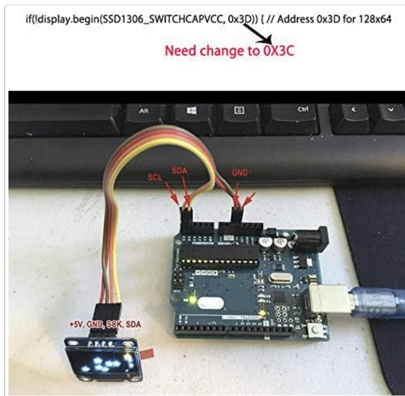
Figure 4: Example wiring of the OLED module with an Arduino board. Note the I2C address change to 0x3C in the code.
