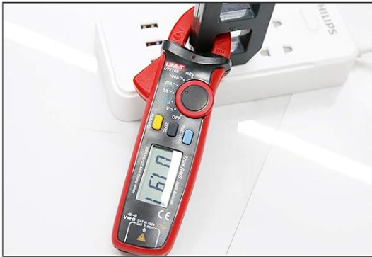
AC current measurement
