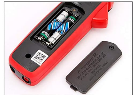
Image: A close-up view of the UNI-T UT210E showing the battery compartment and the test lead input jacks.
