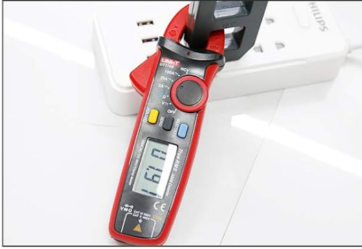
AC current measurement
