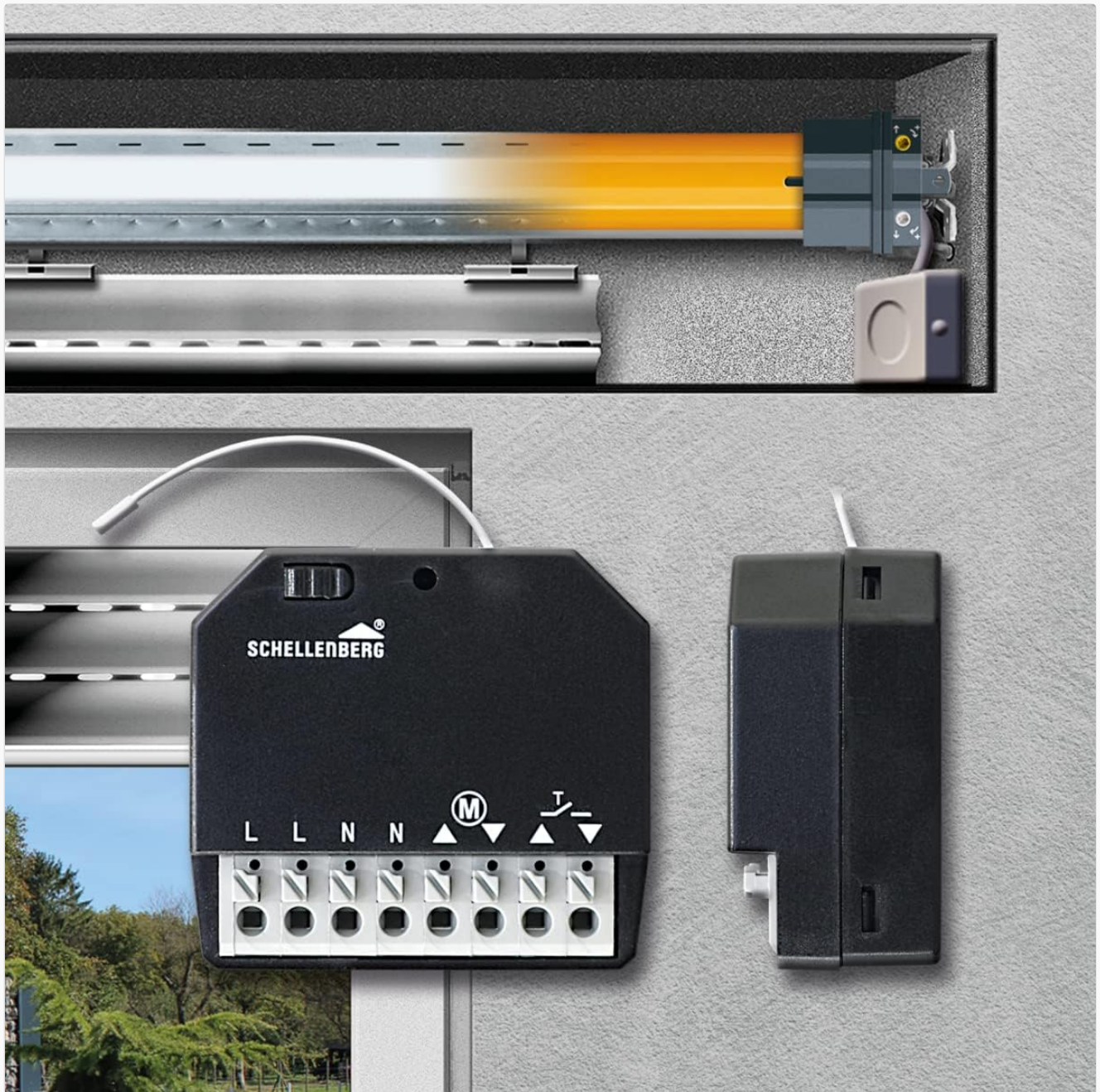
Figure 4: Example Installation. An illustration showing the Schellenberg wireless receiver module installed within the housing of a roller shutter system, with wiring connected to the motor. The module is shown next to a wall-mounted control unit.
