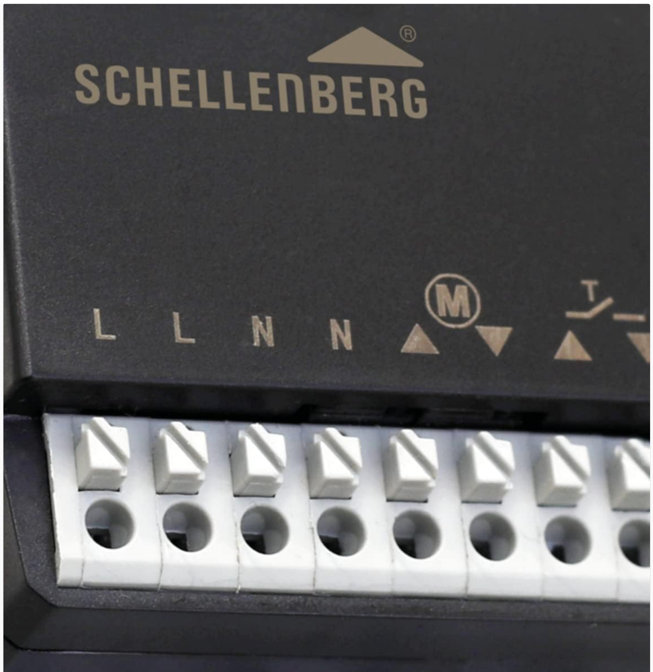
Figure 5: Electrical Terminals. A detailed view of the electrical terminals on the Schellenberg 20018 module, labeled 'L', 'L', 'N', 'N', and motor control symbols, indicating connection points for power and motor wires.
