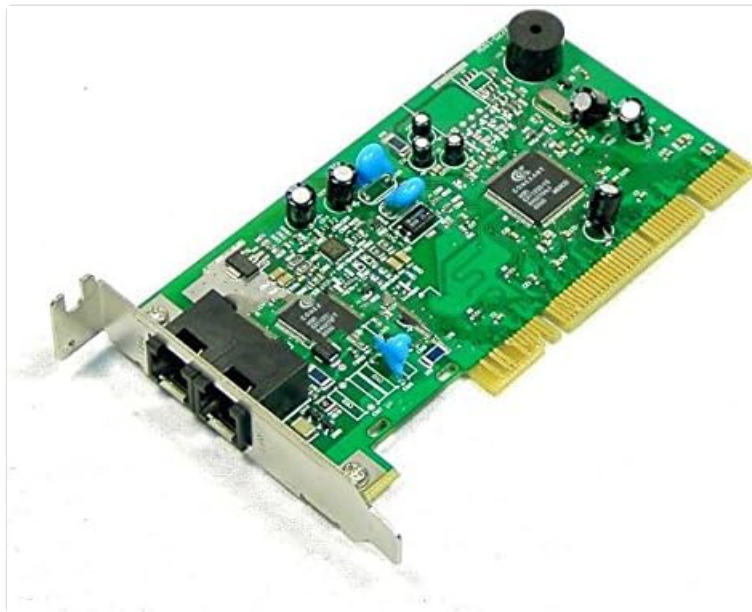
Figure 1: Conexant RD01-D270 PCI Modem Card. This image shows the green circuit board with various electronic components, including capacitors, resistors, and the Conexant chipset. The card features two RJ-11 telephone jacks on its metal bracket for line and phone connections, and a PCI connector at the bottom for motherboard integration.
