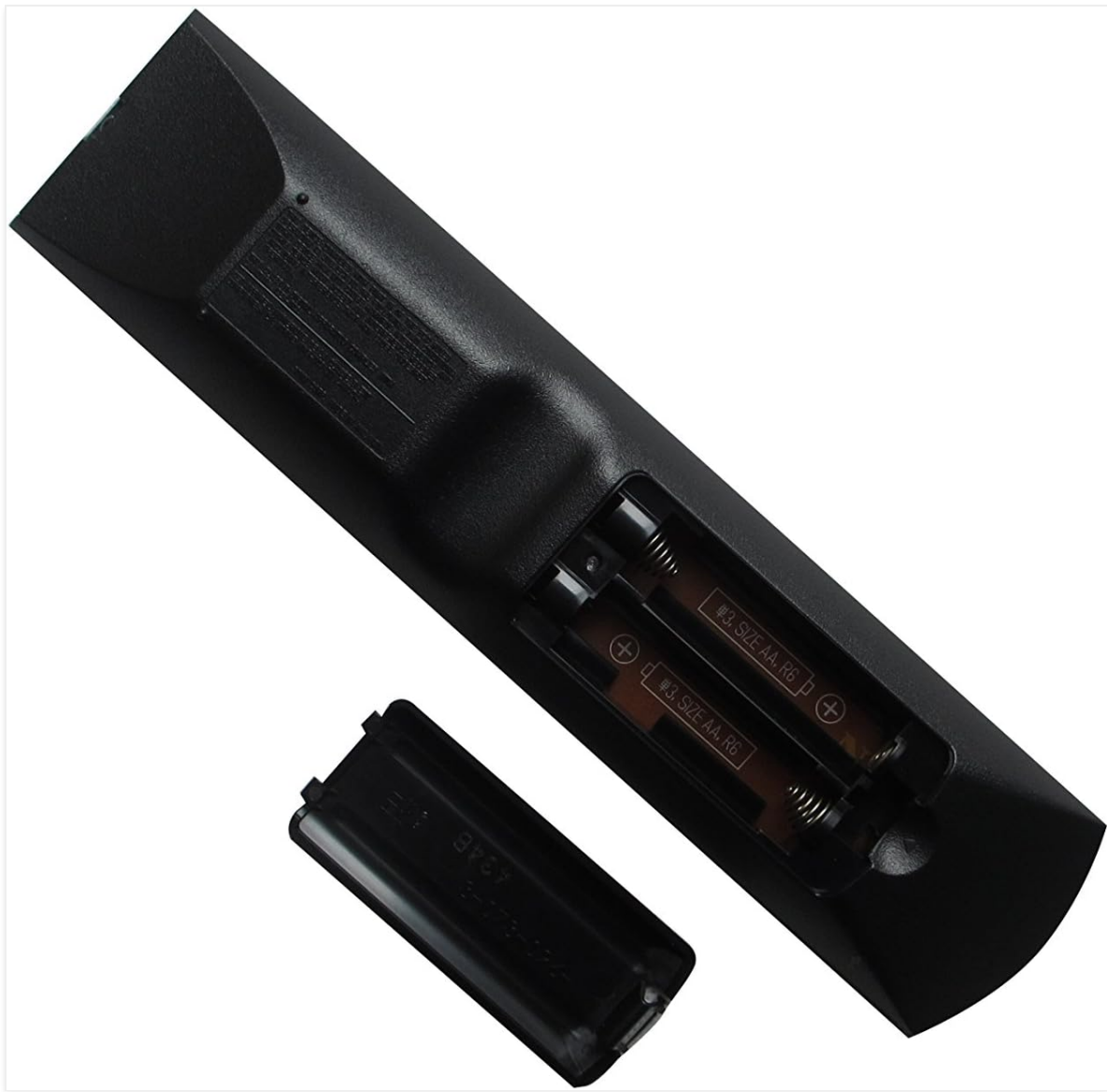
Figure 2: Battery compartment opened, showing battery slots.
