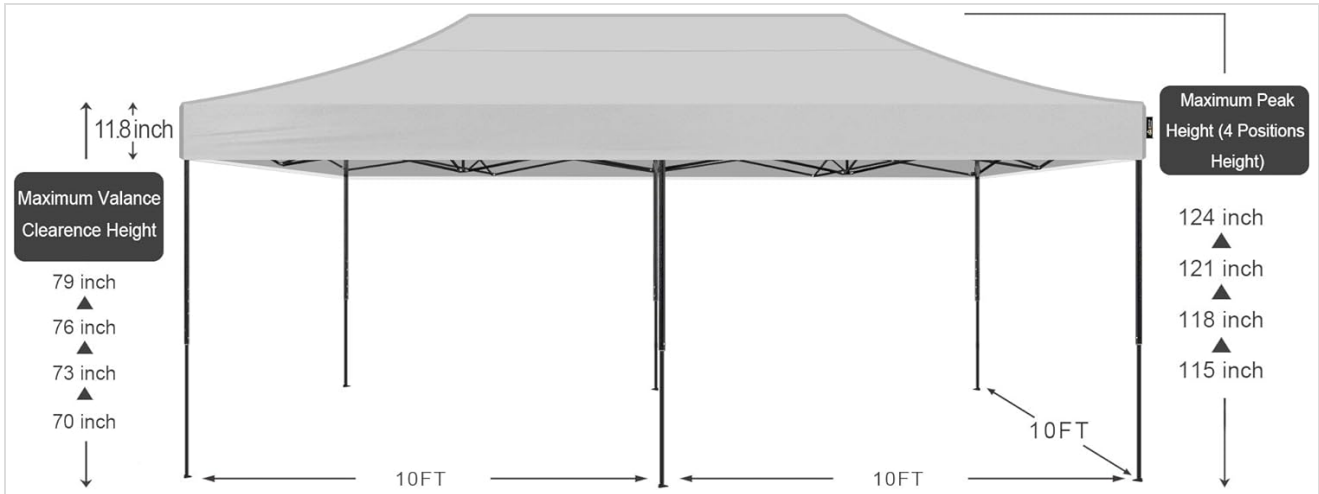
Figure 5.1: Canopy tent dimensions and four adjustable height positions.
