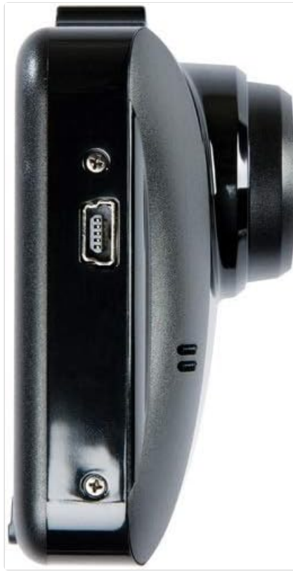
Figure 4.1: Side view of the DrivePro 100, indicating the microSD card slot and emergency record button.
