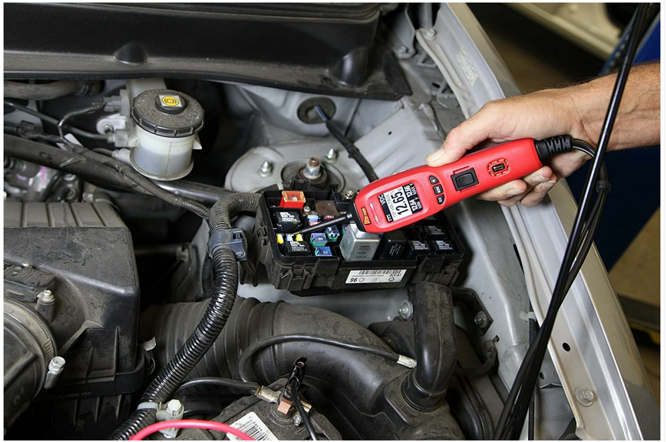
Image 5.4: Testing a fuse for continuity within a vehicle's fuse box.
