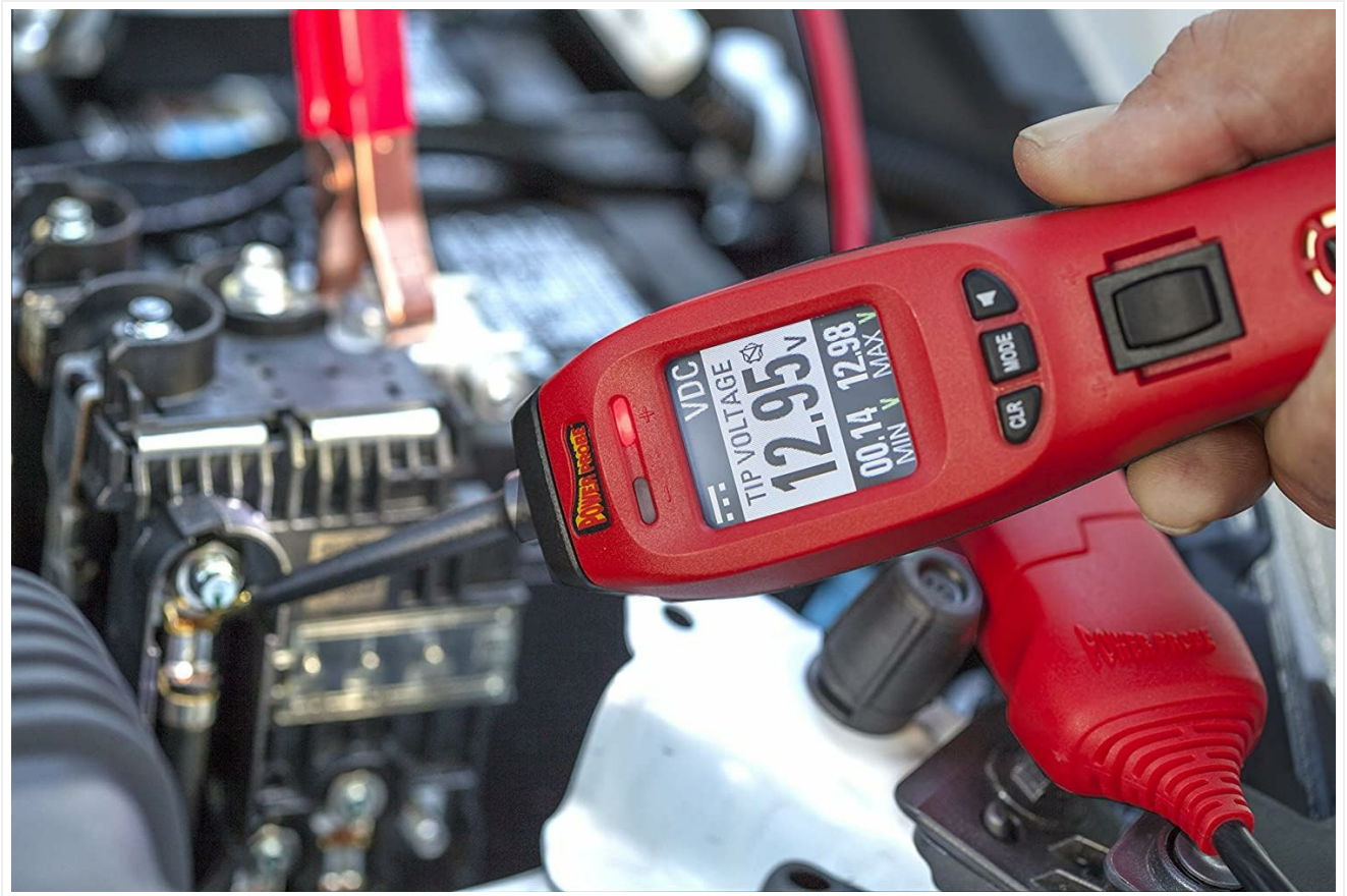
Image 5.3: Using the Power Probe IV to measure voltage at a battery terminal.
