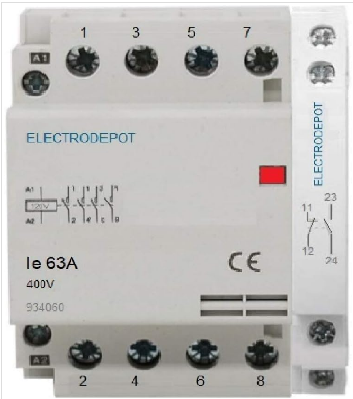
Figure 1: Electrodepot 63A 4-Pole Contactor. This image displays the physical layout of the contactor, showing the main power terminals (1, 3, 5, 7 at the top; 2, 4, 6, 8 at the bottom), the coil terminals (A1, A2), and the auxiliary contact terminals (11, 12, 23, 24). The red indicator light is also visible.
