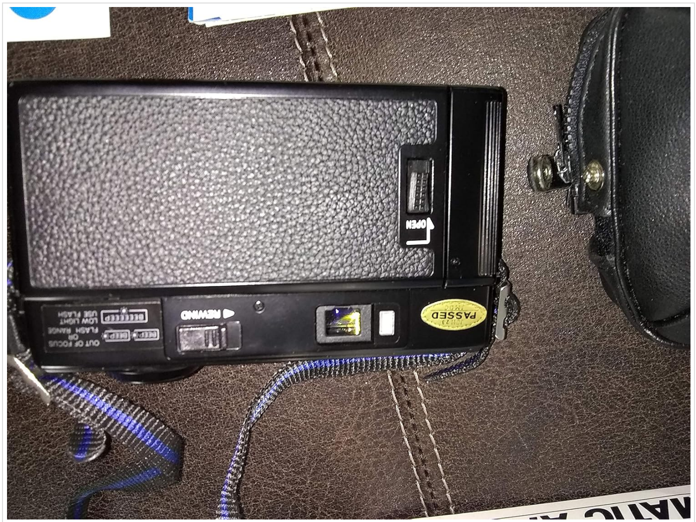
Image: Rear view of the Minolta Hi-matic AF2-M camera, illustrating the film door latch and film rewind switch. This view is crucial for understanding film loading and unloading procedures.
