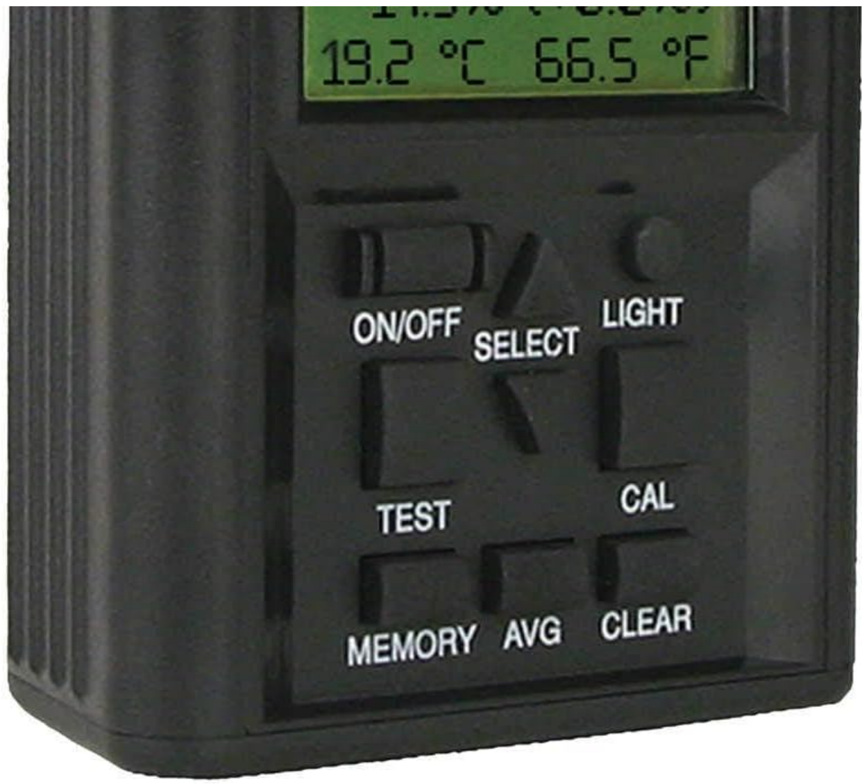
Figure 3: The digital display of the MT-Pro, showing a moisture reading of 14.3% and temperature in both Celsius and Fahrenheit.
