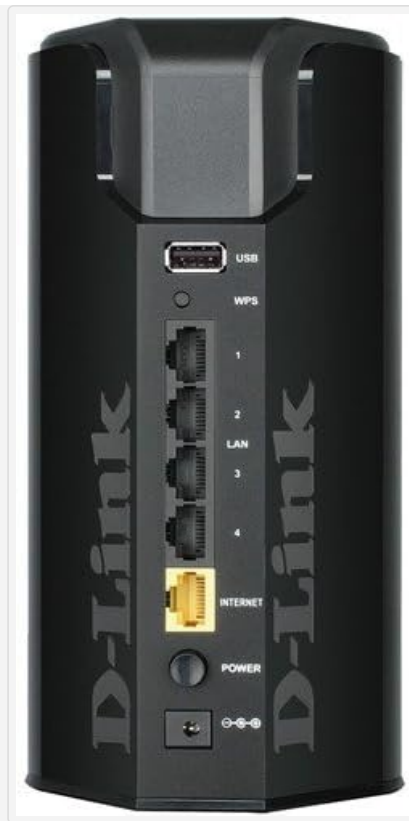
Figure 3.2: Rear view of the D-Link DIR-866L router. This image displays the various ports and buttons, including the USB port, WPS button, four LAN ports, Internet port, power button, and power input.
