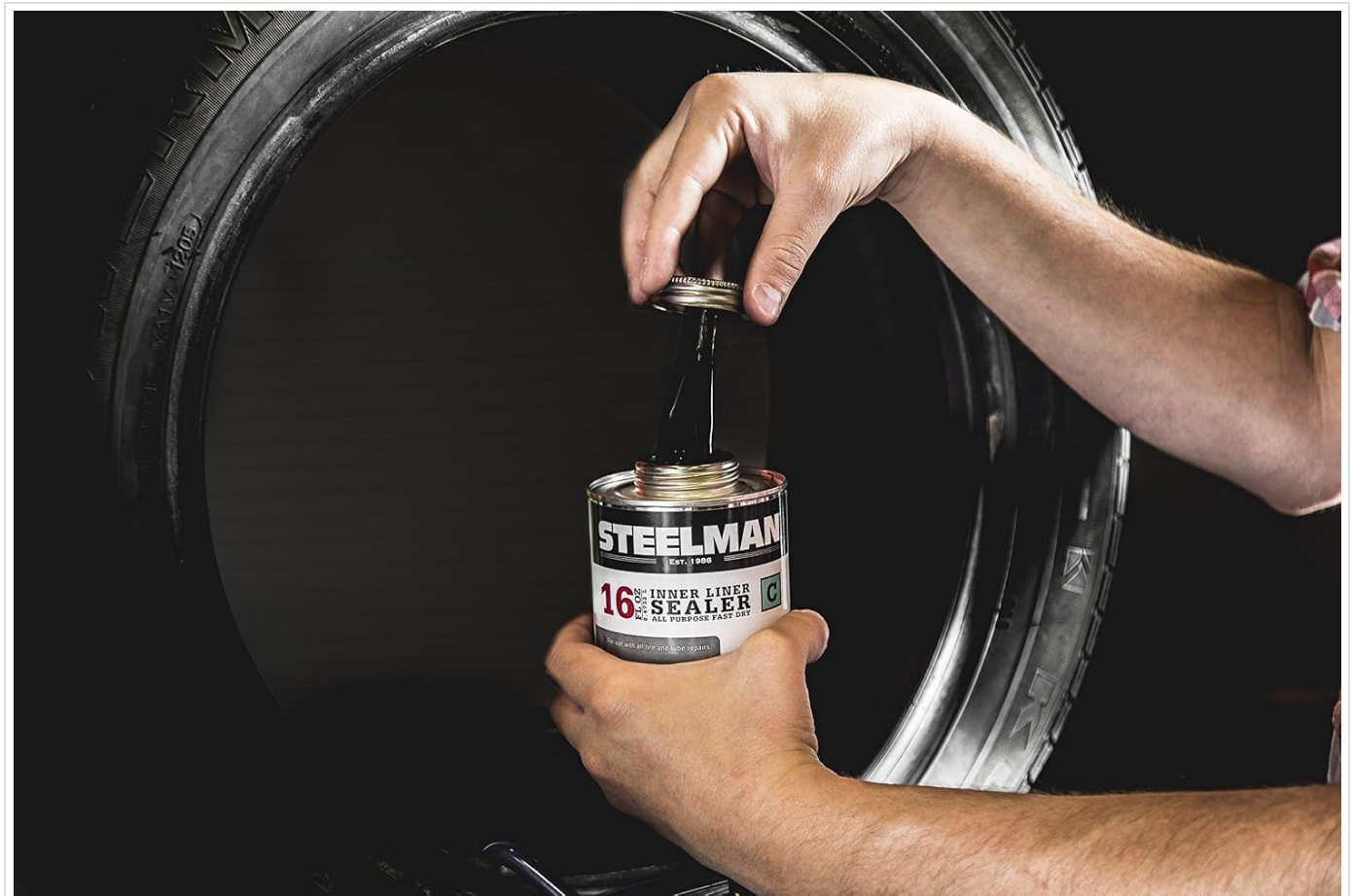
Figure 2: Applying Steelman Inner Liner Sealer to the inner liner of a tire.
