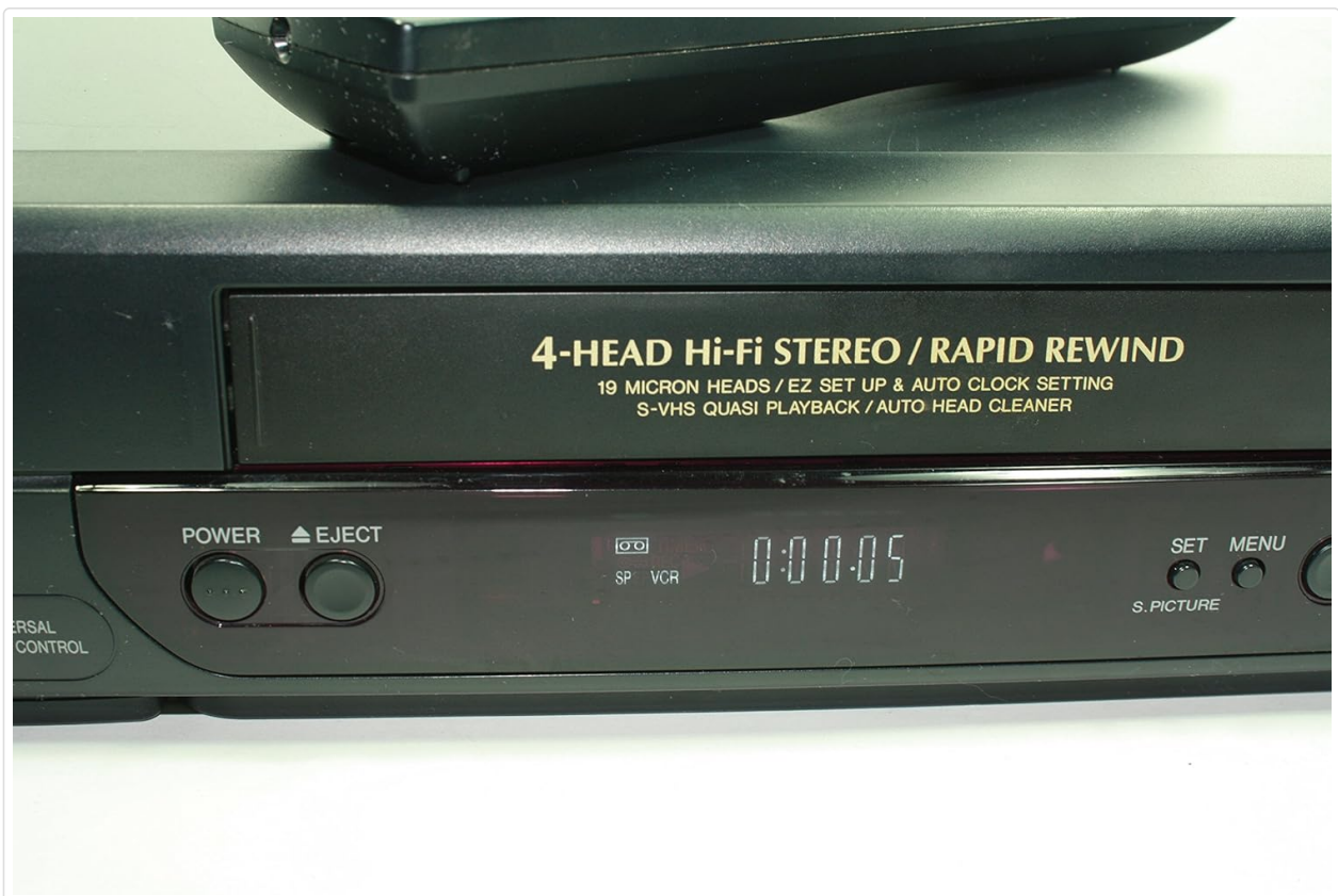
Image 3: A detailed view of the VCR's digital display, showing '0:00:05' which typically indicates tape counter or time. Indicators for SP (Standard Play) and VCR mode are also visible.
