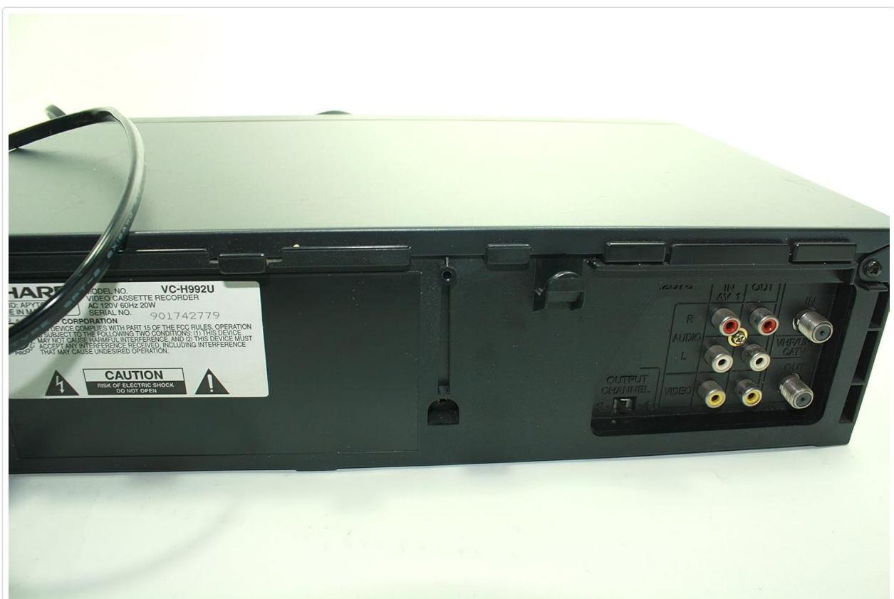
Image 4: The rear panel of the Sharp VC-H992U VCR, displaying various input and output ports. These include RF IN/OUT (VHF/UHF/CATV), Video IN/OUT (RCA yellow), and Audio IN/OUT (RCA white/red for Left/Right stereo). A product label with model number VC-H992U and serial number is also visible.
