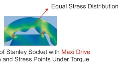
Image: A diagram illustrating the Maxi Drive feature, showing how torque load is redirected away from the corners and applied to the flats, relieving stress points compared to conventional sockets.
