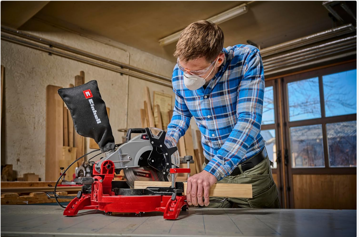
Figure 2.2: A user demonstrating the proper stance and operation of the miter saw for cutting a wooden workpiece.
