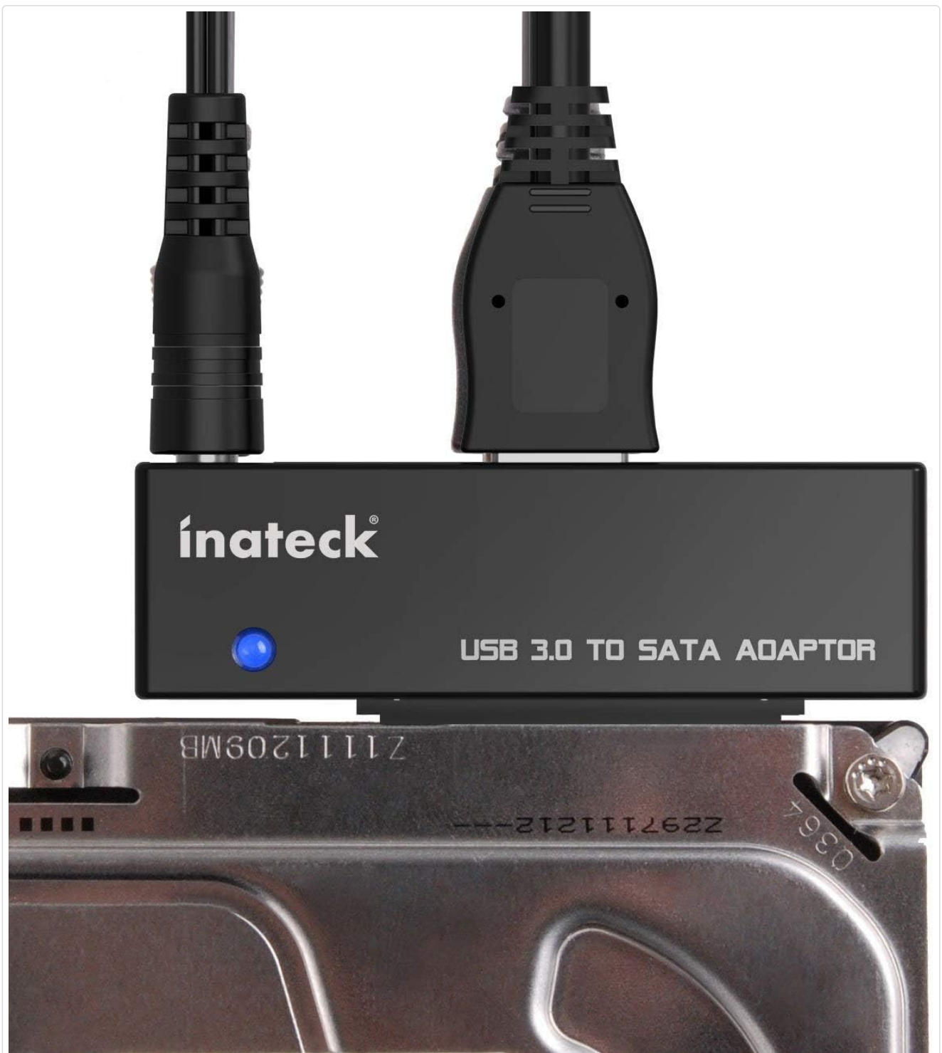
Image: A hard drive being connected to the SATA interface of the Inateck USB 3.0 to SATA Adapter.
