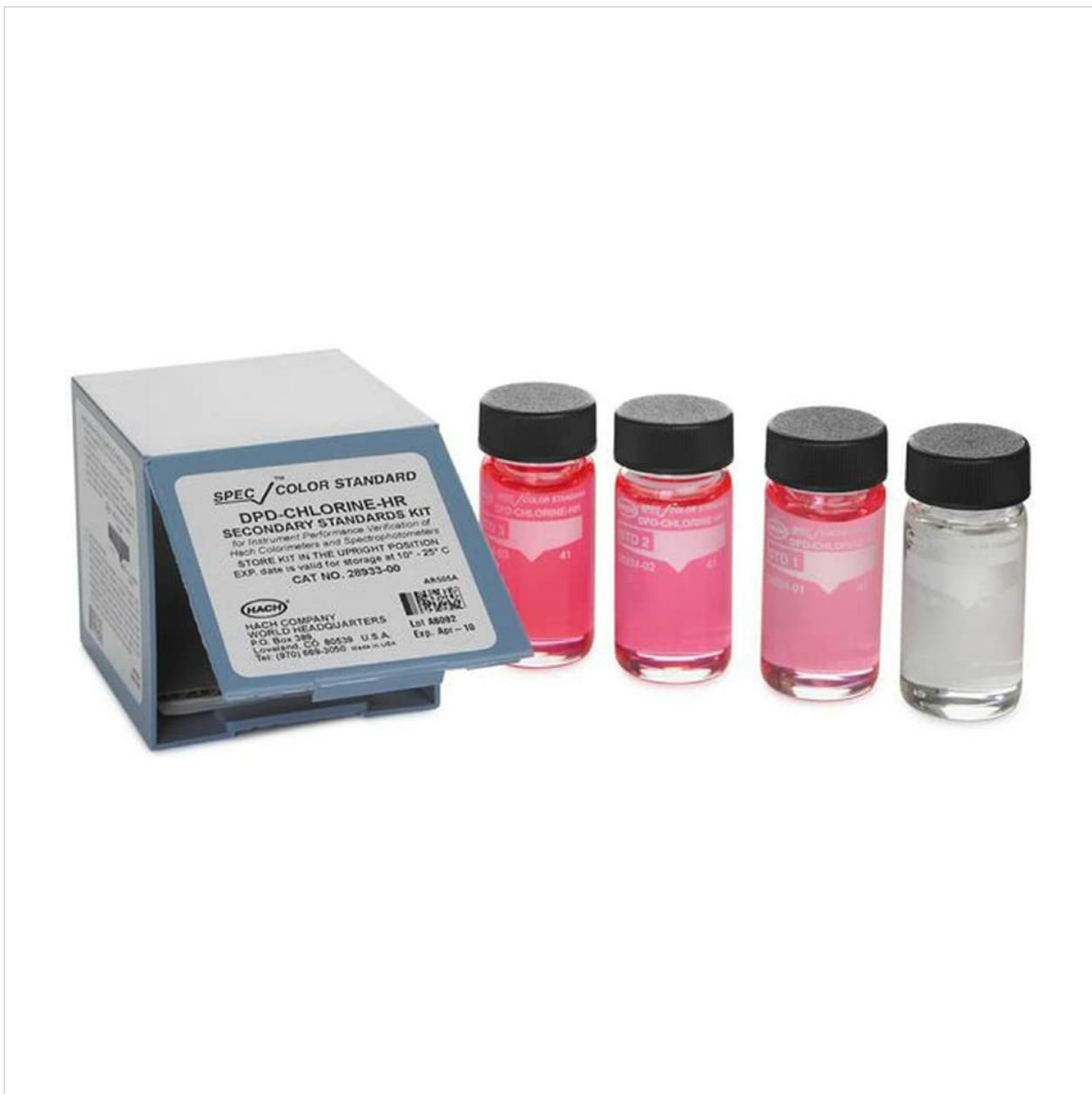
An image showing the Hach SpecCheck Secondary Gel Standards Set. The set includes a white and blue cardboard box labeled 'SPEC/COLOR STANDARD DPD-CHLORINE-HR SECONDARY STANDARDS KIT' and four small glass vials. Three vials contain a pink gel, labeled 'STD 1', 'STD 2', and 'STD 3'. The fourth vial contains a clear or white gel, likely a blank or zero standard. The box also displays the Hach Company logo and contact information.
