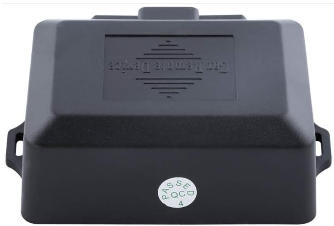
Figure 2.2: Dimensions of the EWC-4 Module. The module measures approximately 78mm in length, 59mm in width, and 30mm in height, indicating its compact size for discreet installation.
