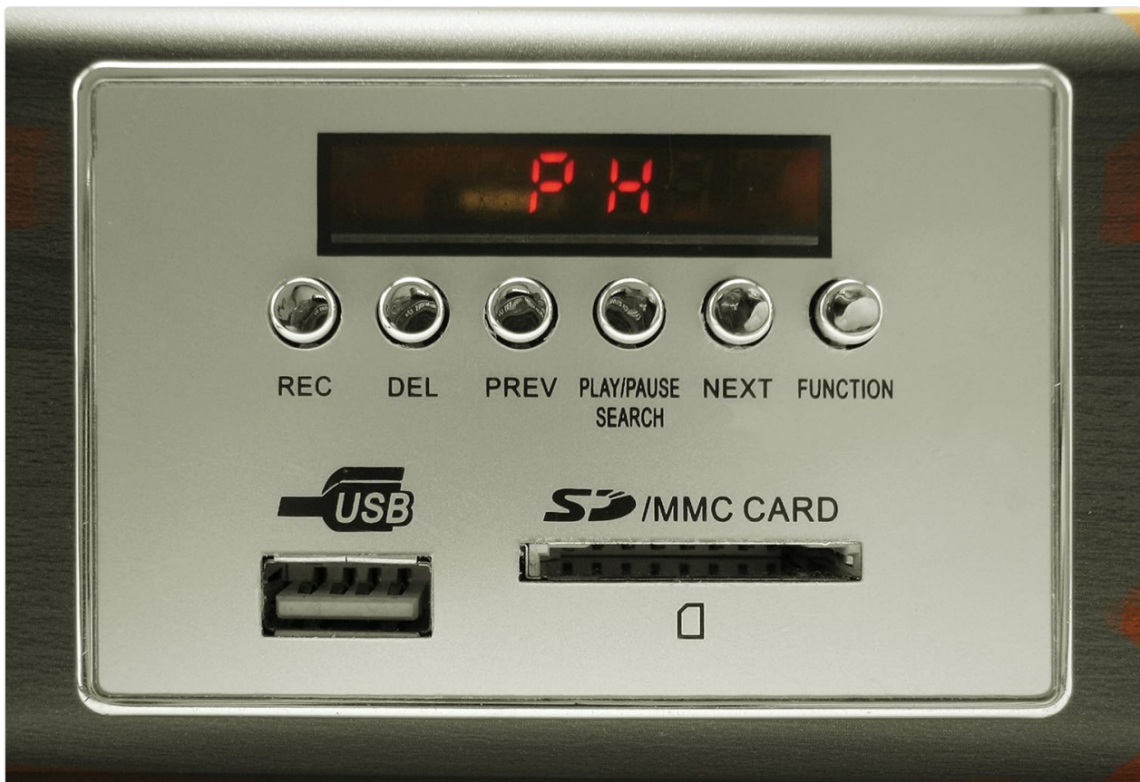
Figure 3.1: Detailed view of the control panel, showing buttons and media slots.
