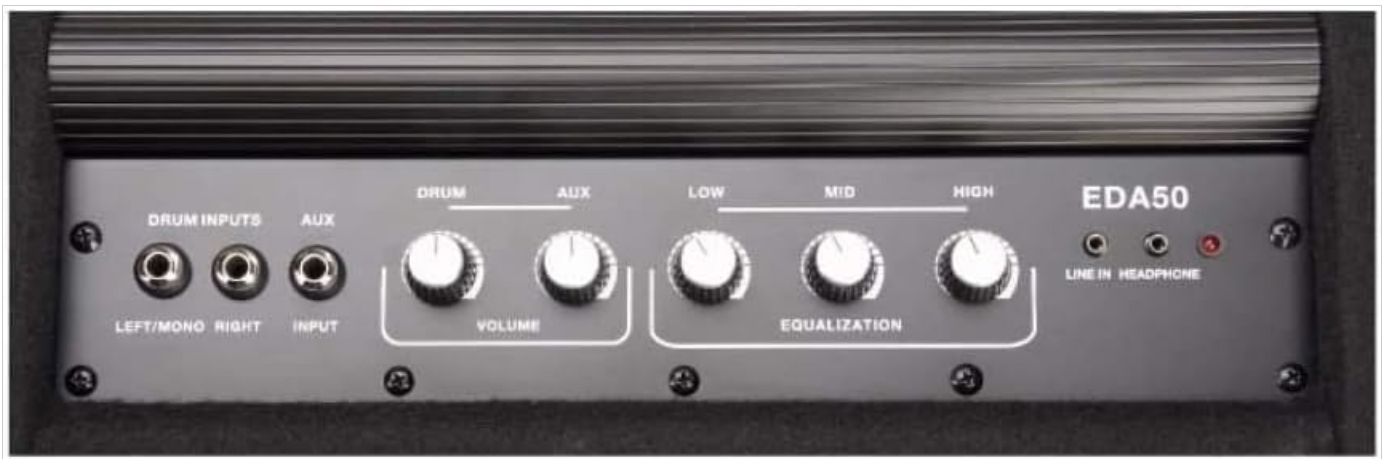
Figure 4.2: Top control panel of the Carlsbro CEDA50XXX, detailing input jacks, volume, and equalization controls.
