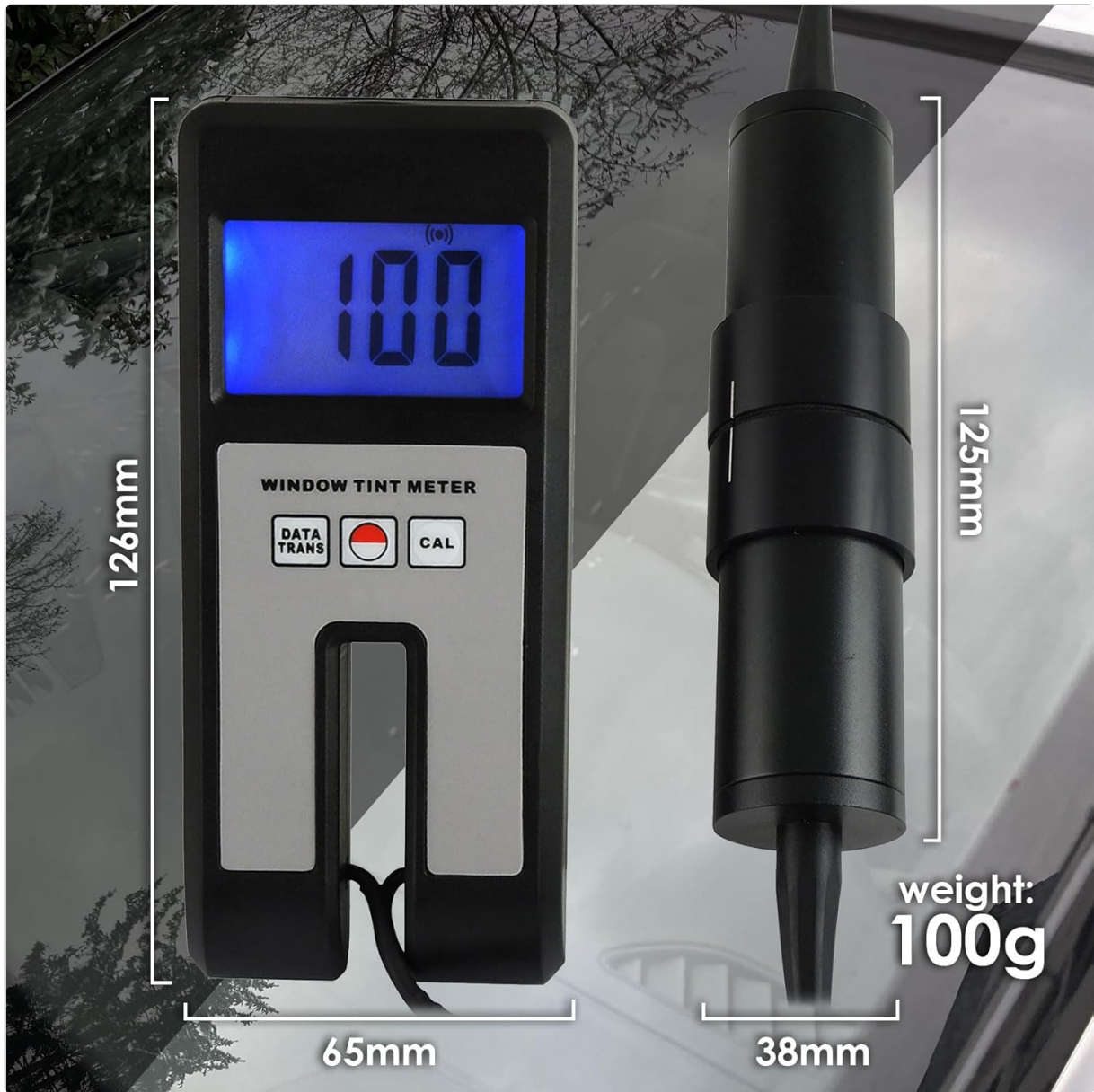
Figure 7.2: Dimensions. This image shows the physical dimensions of the main unit and the probe.
