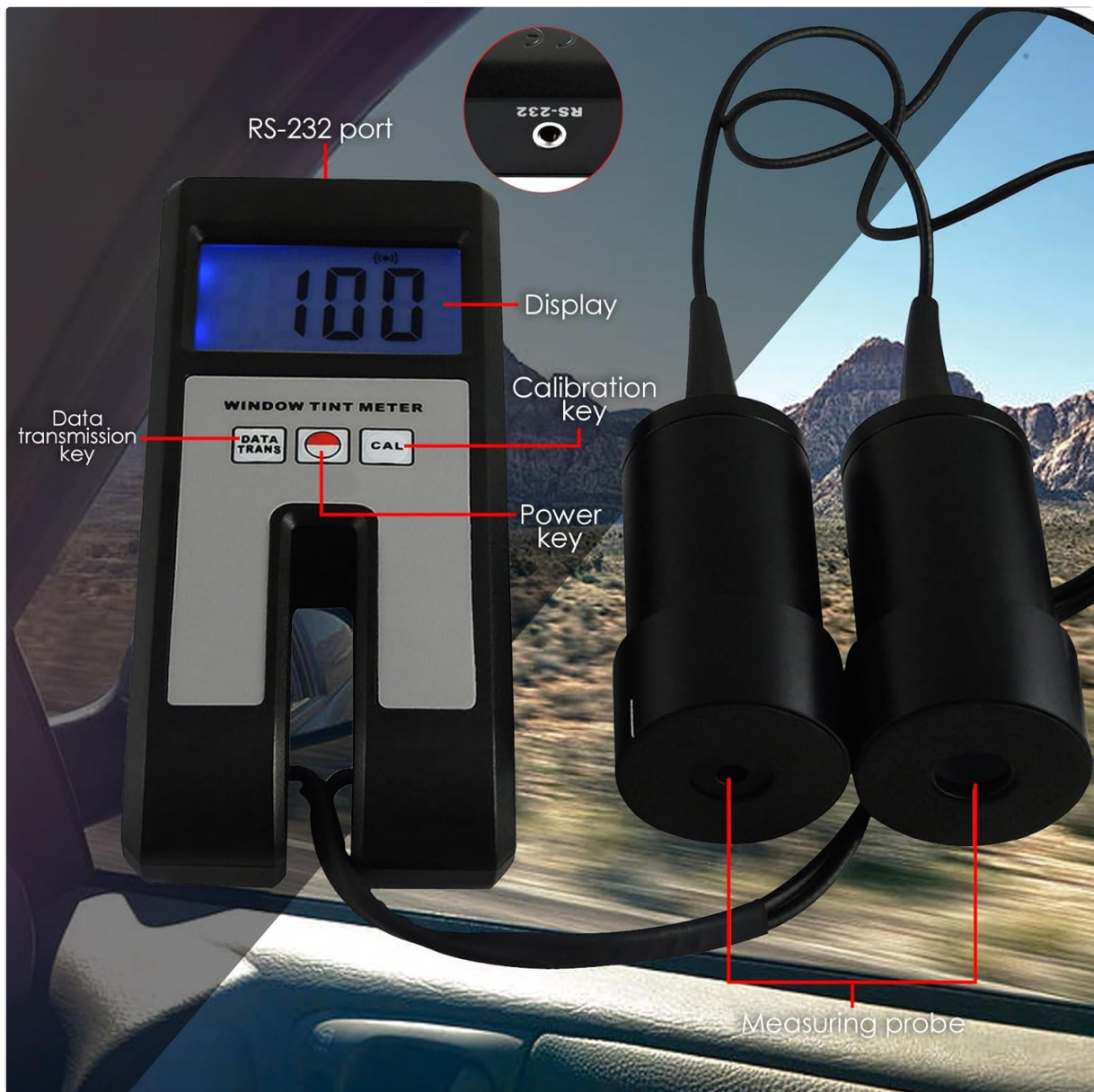
Figure 2.2: Labeled components of the WTM-1100 Tint Meter. This image identifies the RS-232 port, display, calibration key, power key, and measuring probes.
