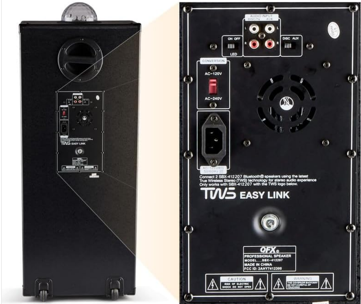
Image: Detailed view of the QFX SBX-412207BT speaker's back panel, showing the audio input ports (RCA, Aux), LED switch, AC voltage conversion switch (120V/240V), and power input.
