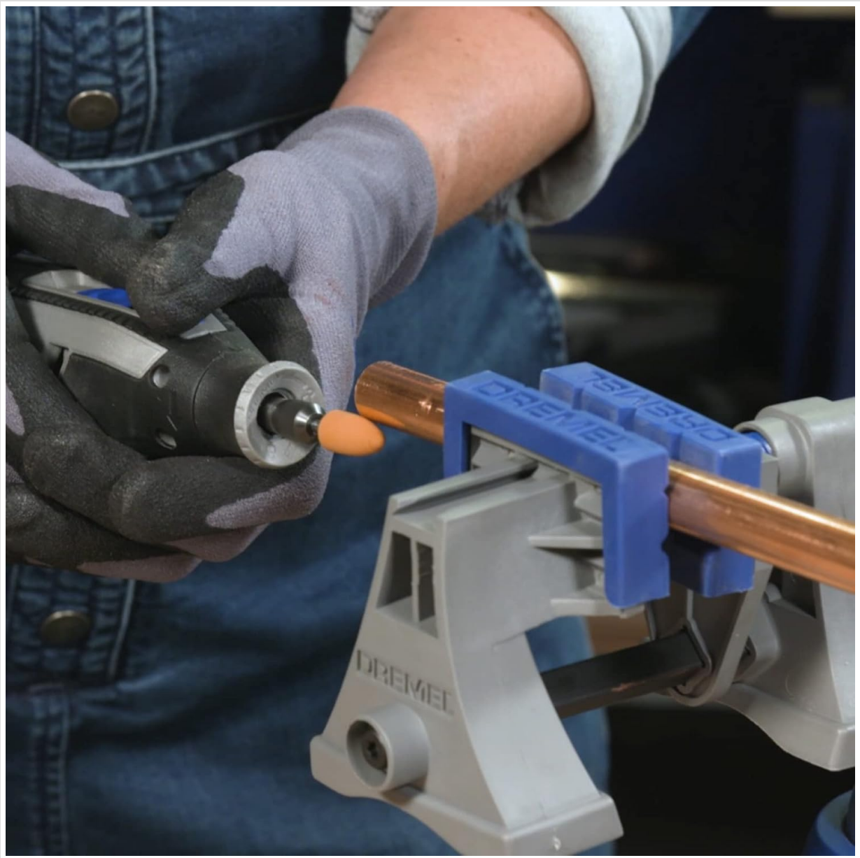
Image: A close-up view demonstrating the attachment and use of a grinding accessory on a Dremel rotary tool, working on a copper pipe.
