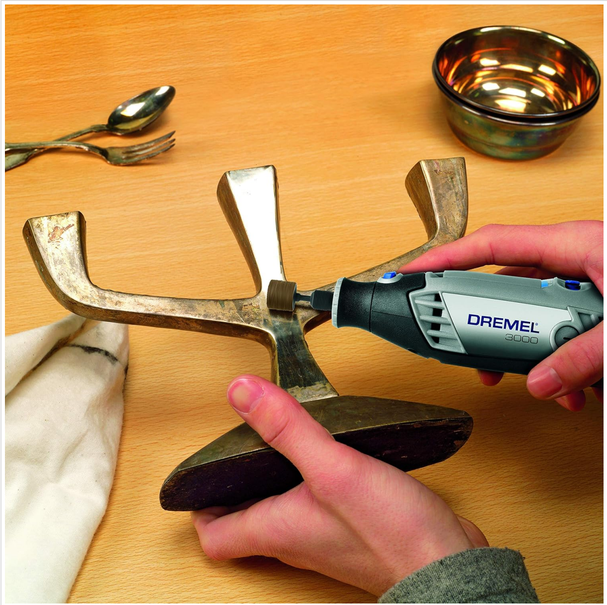
Image: A Dremel rotary tool fitted with a grinding stone, actively being used to refine the surface of a metal component.
