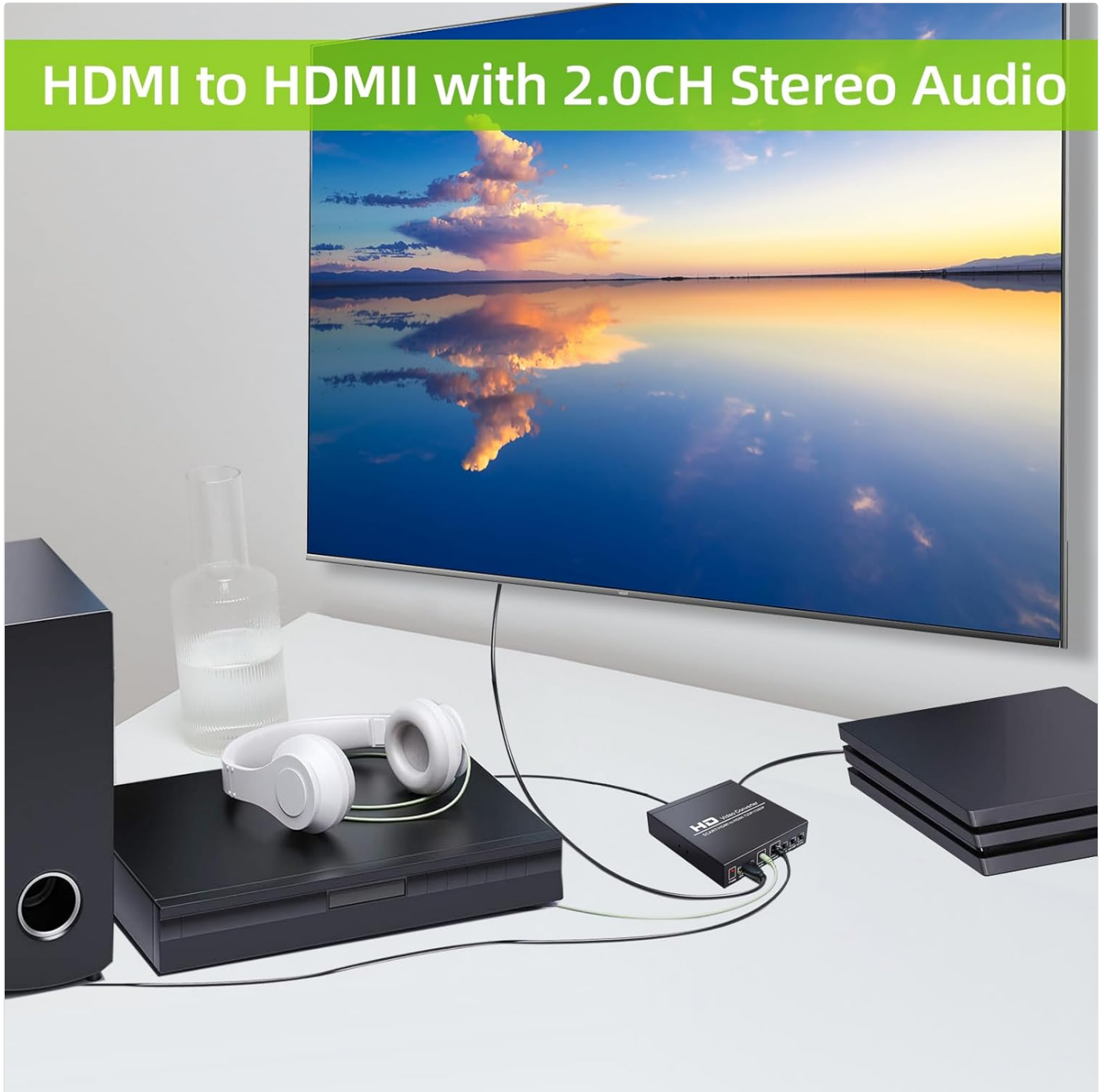
Figure 5: Example of HDMI input and audio output connections.
