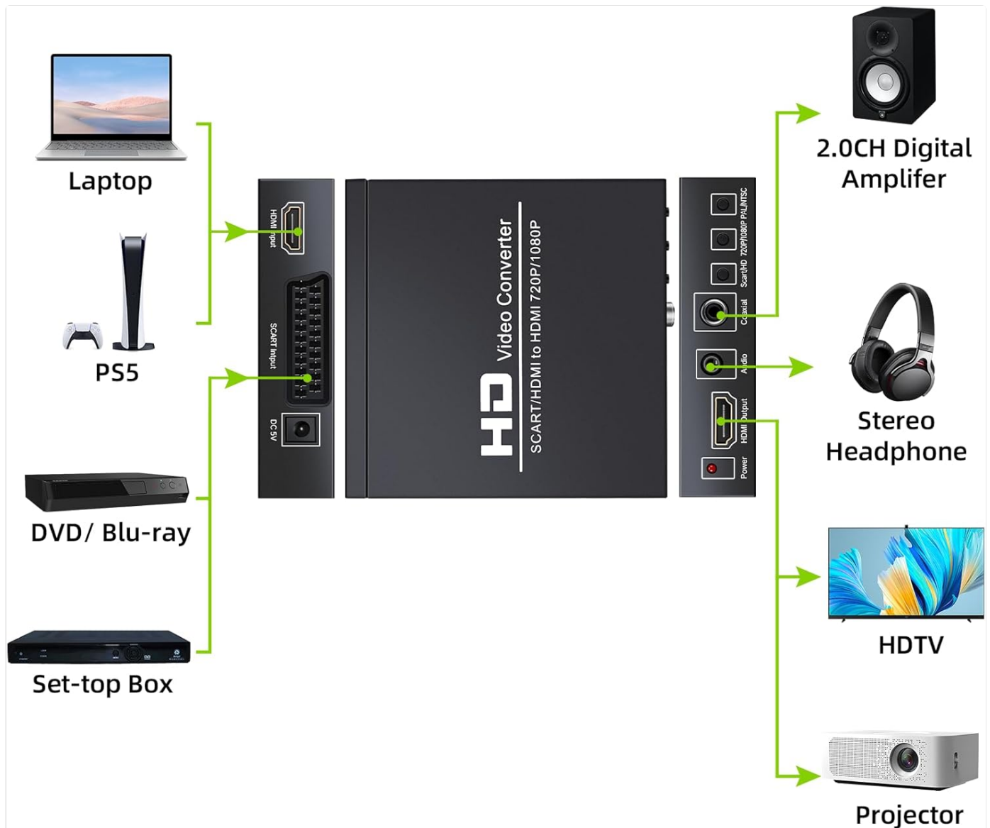
Figure 3: Connection diagram for various input and output devices.
