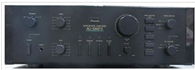
Figure 1: Front view of the SANSUI AU-D607X Integrated Amplifier. The amplifier is black with various knobs, buttons, and switches on its front panel, including controls for input selection, tone adjustments, volume, and speaker output.
