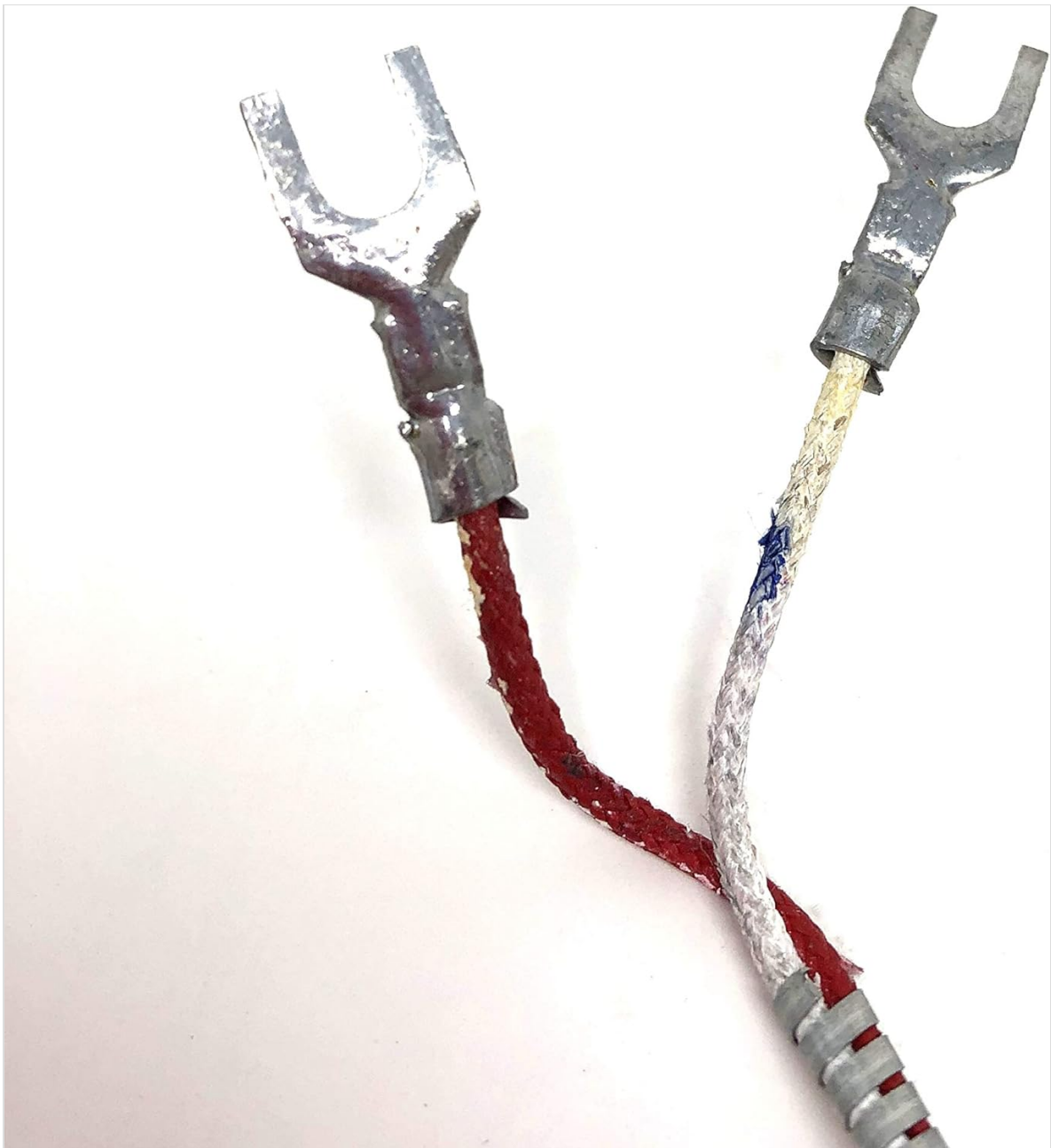
Figure 4: Electrical spade connectors used for wiring the pilot assembly, ensuring a secure connection.
