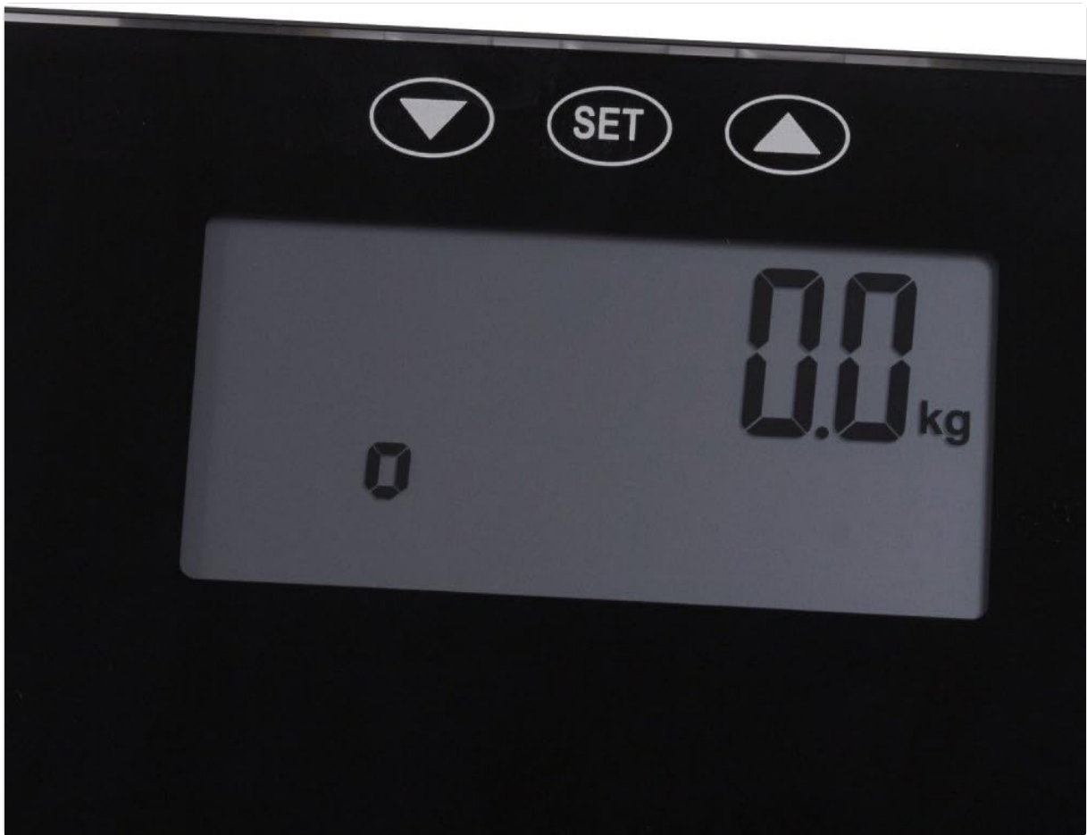
Figure 4.2: Close-up of the digital display showing '0.0 kg' and the 'SET', Up, and Down control buttons.
