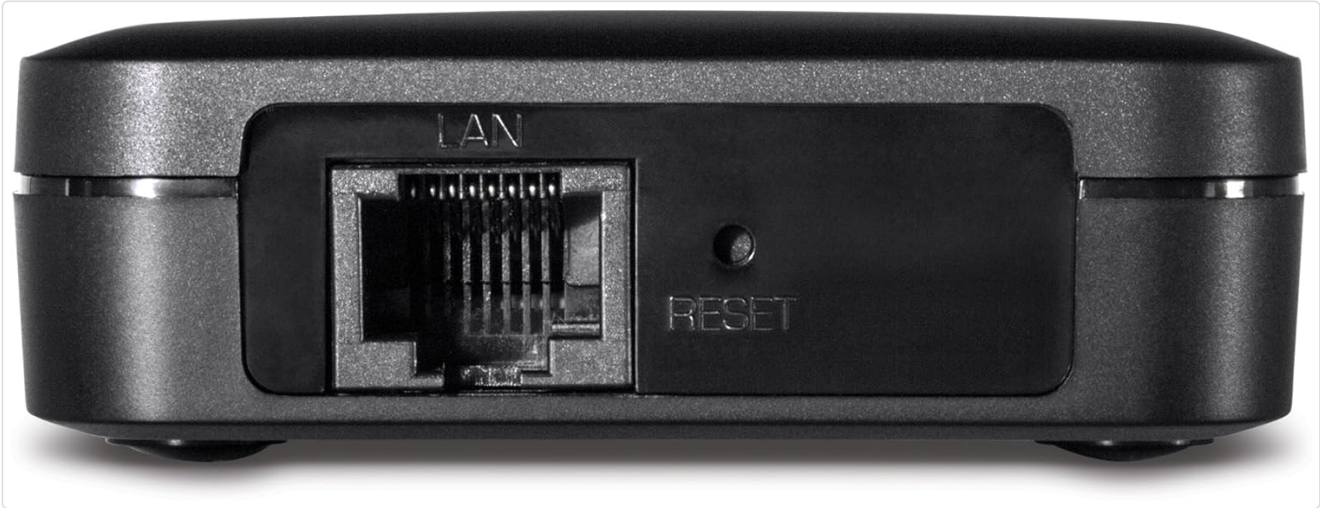
Rear view of the TEW-820AP, highlighting the LAN port and Reset button.
