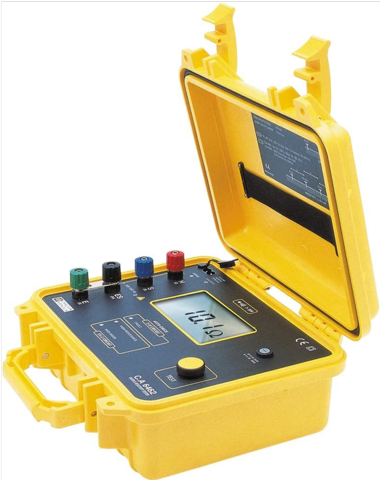
Figure 3.2: Angled View of CA 6462. This image shows the Chauvin Arnoux CA 6462 Grounding Tester from an angled perspective, highlighting its robust yellow carrying case with the lid open. The internal components, including the display and terminals, are visible, along with the sturdy hinges and latches of the case, emphasizing its portability and protection.
