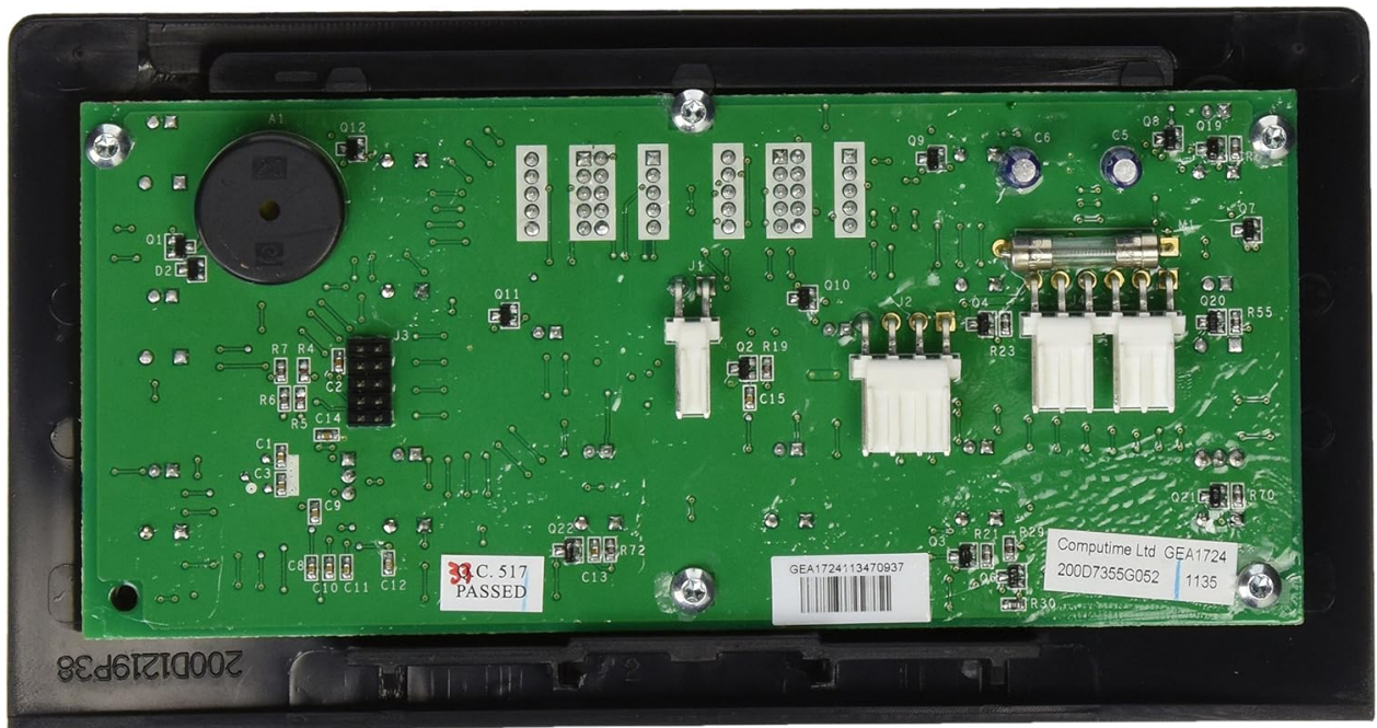
Image: Back view of the circuit board for the dispenser interface assembly, showing various wiring connectors and electronic components.
