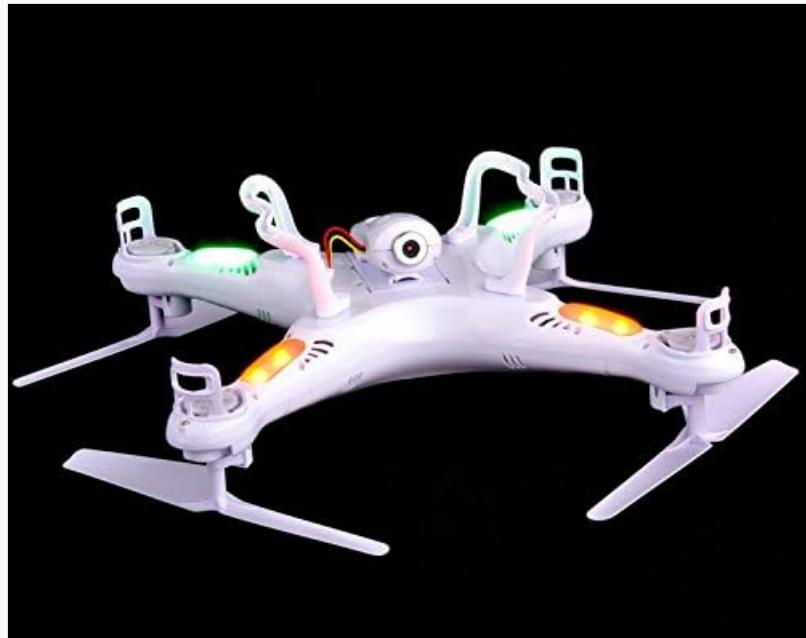
Locate the camera port on the underside of the quadcopter. Gently slide and secure the HD camera into place, ensuring a firm connection. The image above shows the quadcopter with the camera module attached to its underside.
