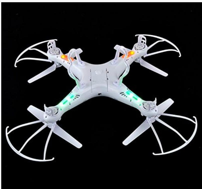
Carefully attach the four protection frames (propeller guards) to the motor arms of the quadcopter. Then, attach the two landing skids to the underside of the main body. Use the provided screwdriver if necessary. The image above illustrates the quadcopter with its propeller guards installed.
