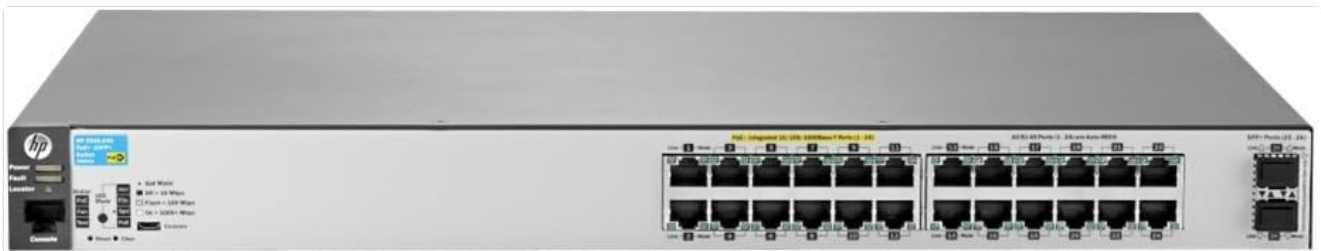
Figure 1: Front Panel of HP J9854A Switch. This image displays the front panel of the HP 2530-24G-PoE+-2SFP+ Switch. On the left, the HP logo, power, fault, and locator LEDs are visible, along with a console port. The center features 24 RJ-45 Gigabit Ethernet ports, each with Link/Activity and PoE status indicators. On the right, two SFP+ ports are present for high-speed uplinks.
