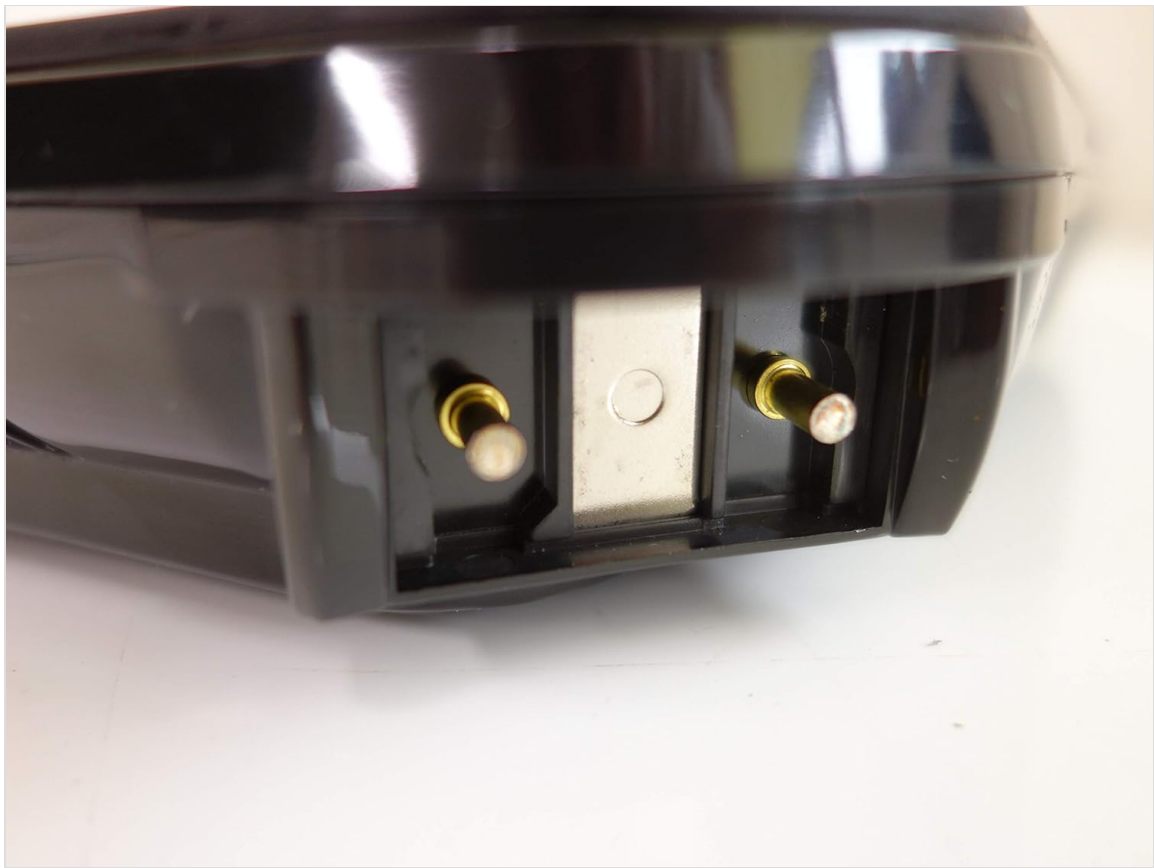
Figure 3.2: The power input port on the IH Cooker where the detachable cord connects.
