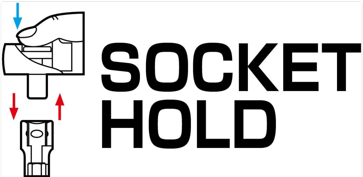
Figure 2: Socket Hold Mechanism. This diagram visually explains the process of attaching and detaching sockets using the quick-release button.
