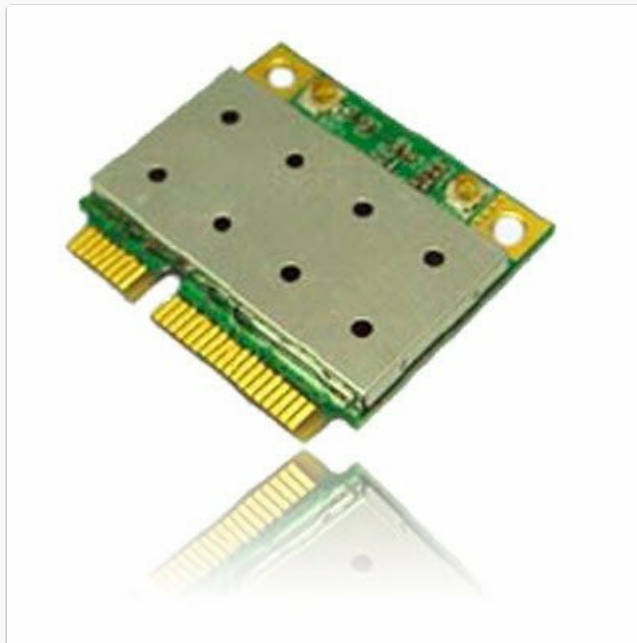
Image of the Azurewave AW-NB041 PCIe Mini-Card, showing its compact form factor and connectors.
