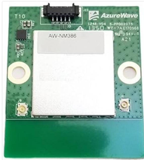
Figure 1: Azurewave AW-NM386 Wireless LAN USB Module. This image shows a green circuit board with a silver metallic shield covering the main chip, labeled 'AW-NM386'. It features a black connector at the top and two circular mounting holes, one on each side. The AzureWave logo and other technical markings are visible on the board.
