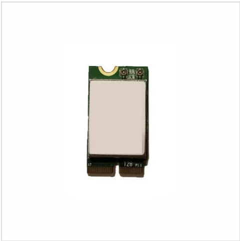
Figure 1: Azurewave AW-NB136NF WiFi and Bluetooth 4.0 NGFF (M.2) module. This image displays the Azurewave AW-NB136NF module, a compact NGFF (M.2) card designed for wireless connectivity. It features two antenna connectors at the top and the M.2 interface at the bottom, indicating its form factor for integration into compatible devices.
