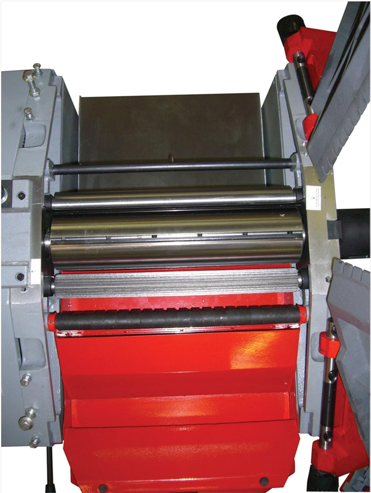
Figure 2: Close-up view of the infeed and outfeed rollers and the blade area, crucial for smooth material processing.
