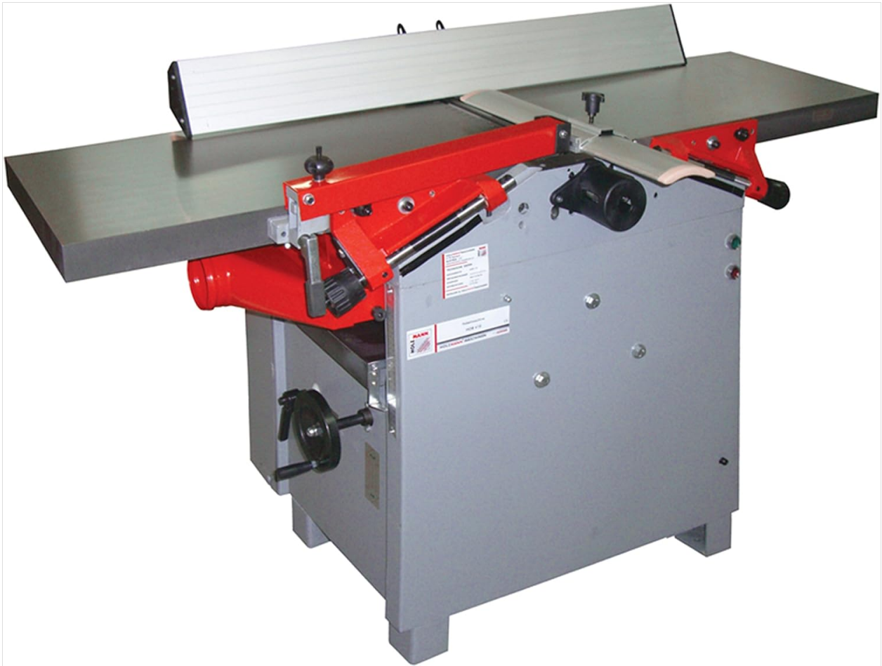
Figure 1: Main view of the Holzmann HOB410N-400V Planer-Thicknesser, showcasing its robust design and primary components.
