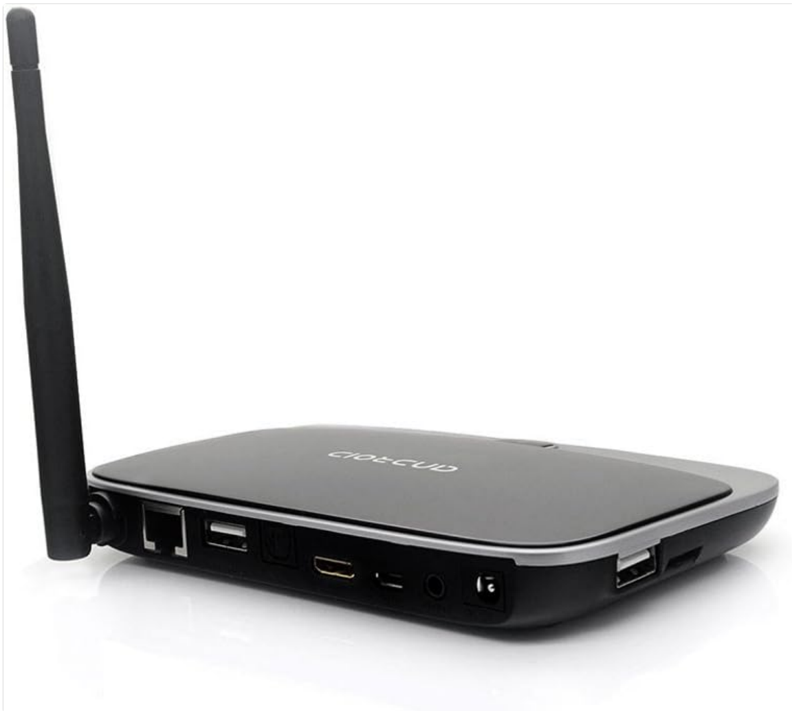
Figure 4.2: Side view of the TV Box, illustrating the available ports for connectivity.
