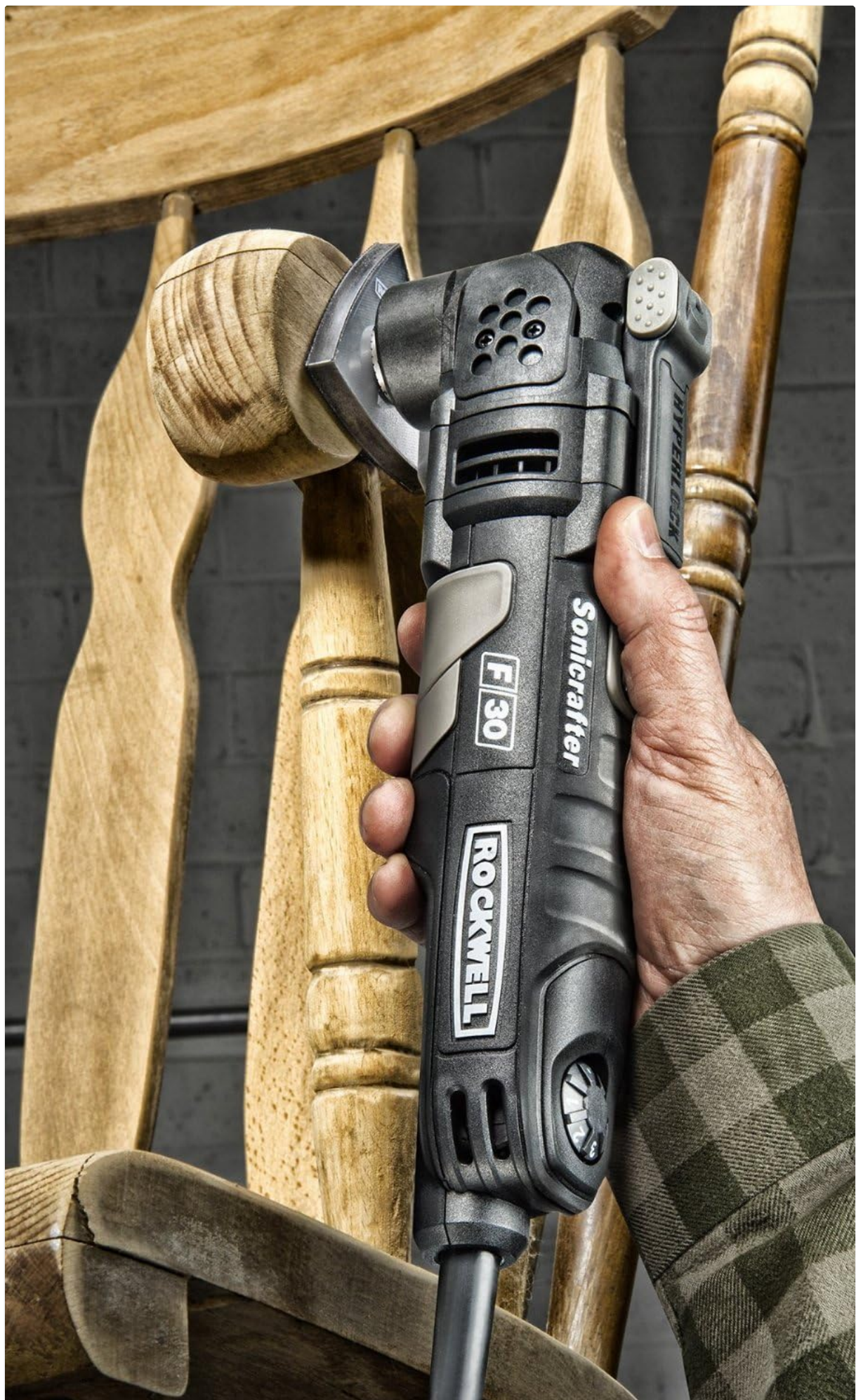
Image 5.7: The multi-tool equipped with a sanding pad, smoothing a wooden chair leg, highlighting its use for finishing tasks.
