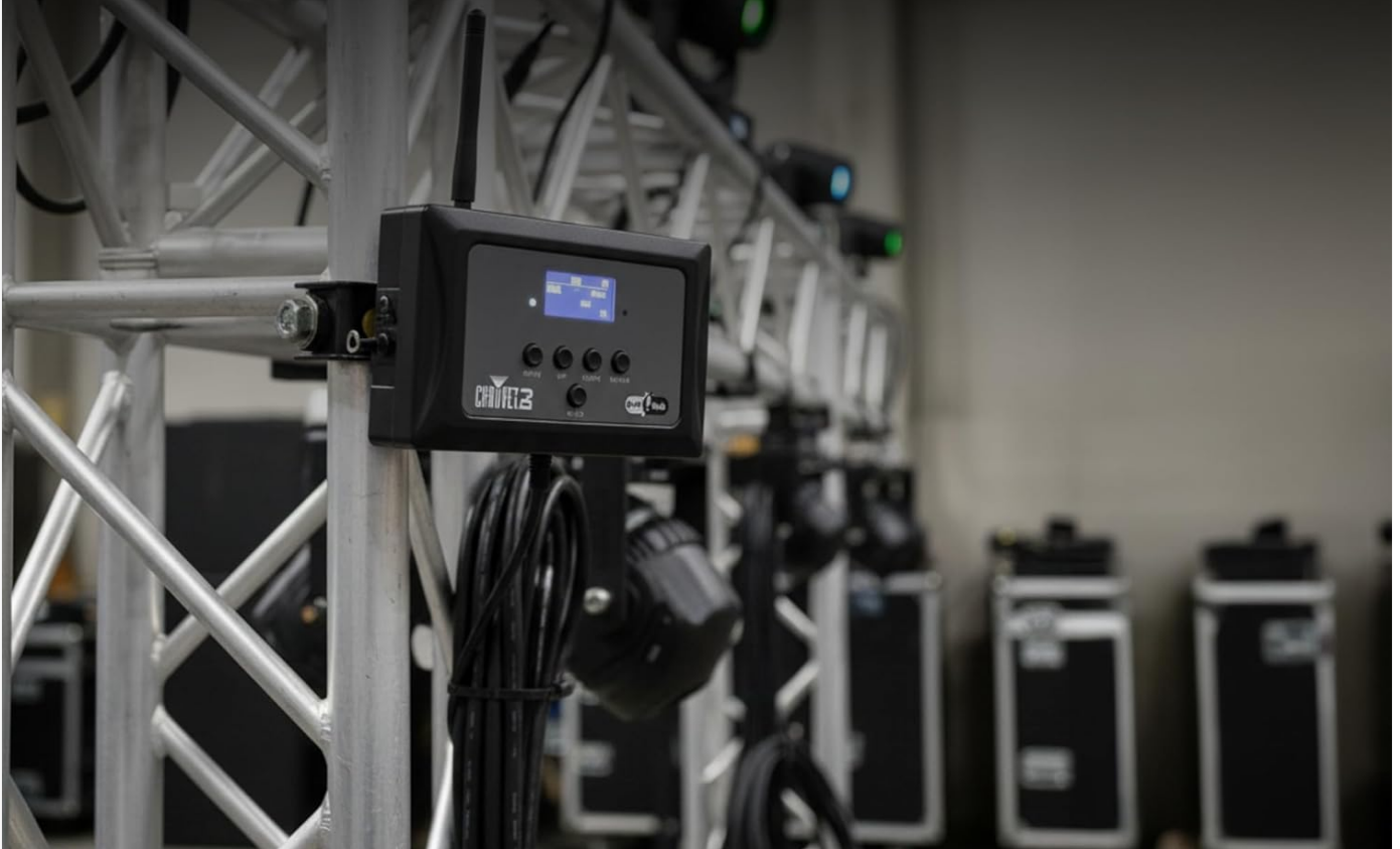
The D-Fi Hub mounted on a truss, demonstrating its application in a professional lighting rig.
