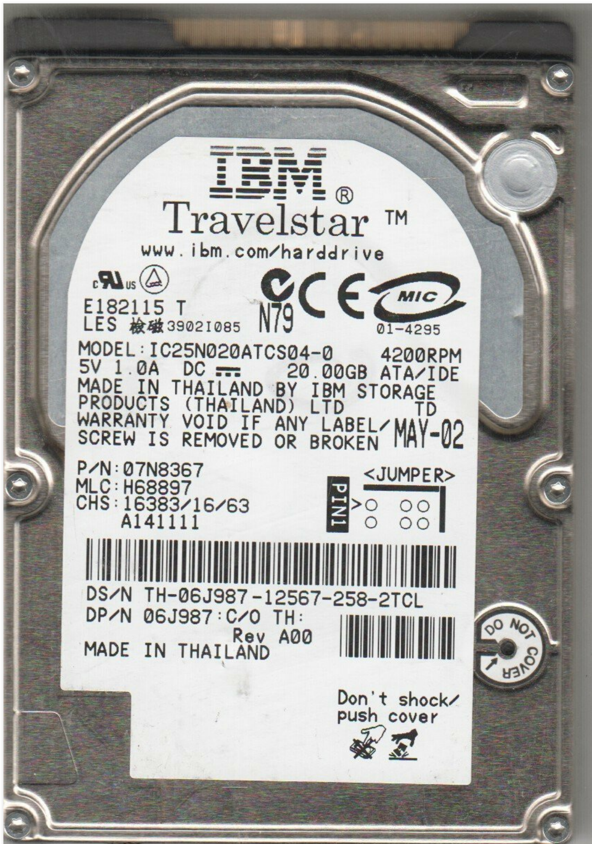
Figure 1: IBM 20GB IDE 2.5 Hard Drive (Model IC25N020ATCS04-0). This image displays the physical appearance of the hard drive, including its label with model and serial numbers, and the IDE connector interface.
