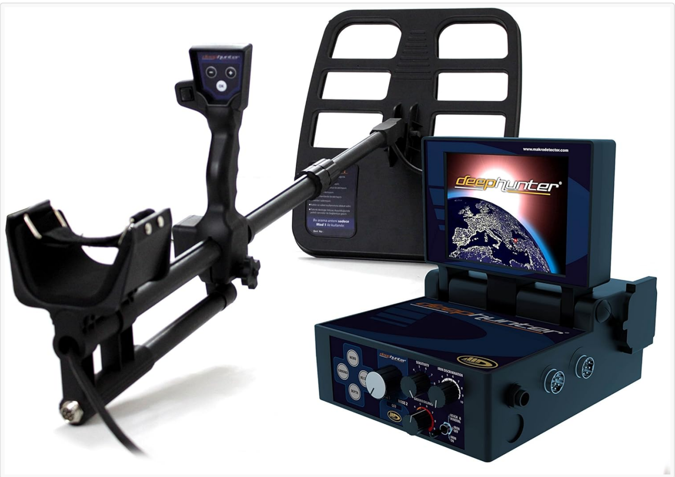
Figure 3.2: The Deephunter Pro detector configured with a large rectangular search coil, ideal for deep treasure hunting.
