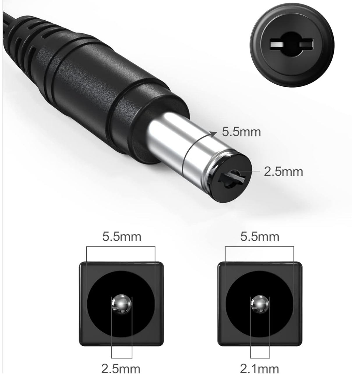
Image 4.2: DC Output Connector. This image provides a detailed view of the DC barrel connector, highlighting its 5.5mm outer diameter and its compatibility with both 2.1mm and 2.5mm inner pin sizes.
