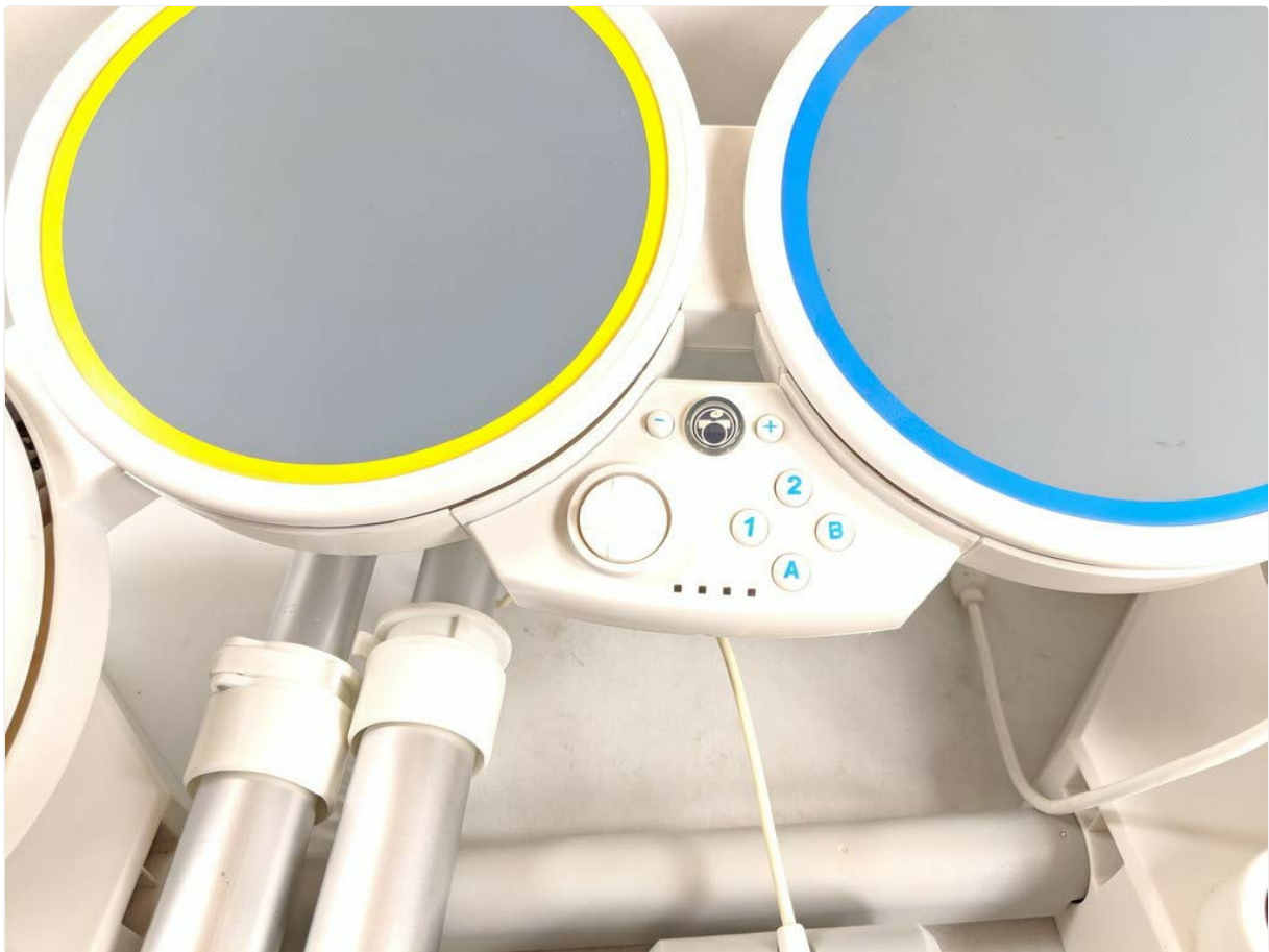
Image 3.1: Central control panel of the drum controller, featuring buttons and the connection interface.
