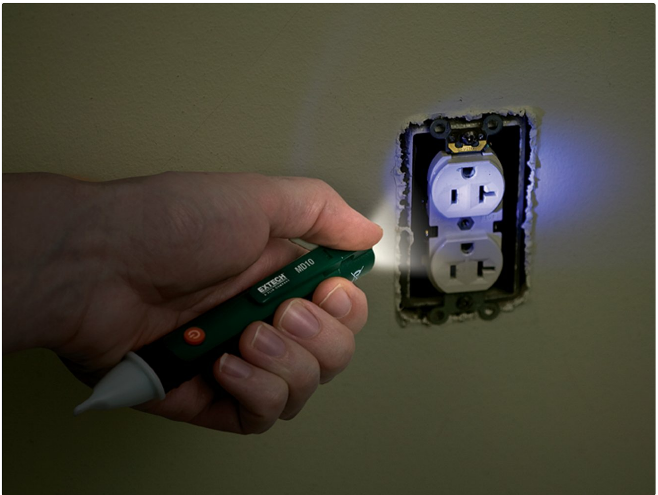
Figure 3: The Extech MD10 being used to illuminate an electrical outlet, demonstrating its built-in flashlight function.
